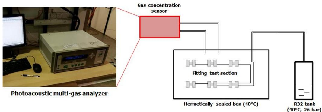
Figure 6: Diagram of leak rate measurement facility.
