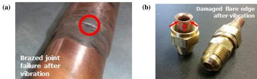
Figure 5: Images of fitting failures during vibration testing: (a) Braze joint and (b) flare fitting.
