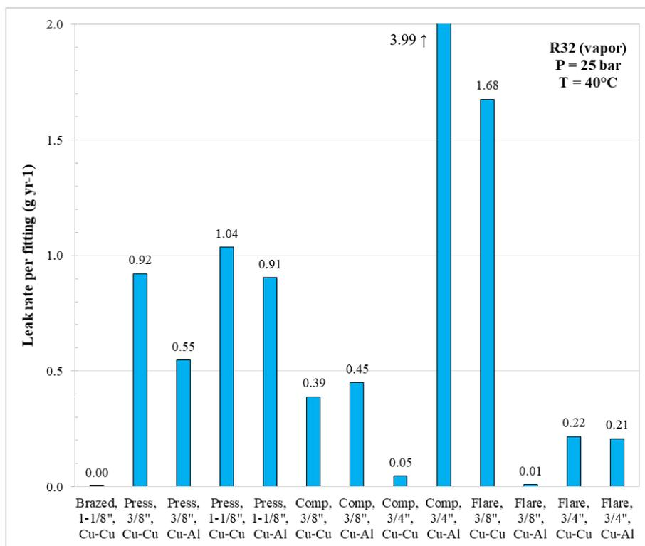
Figure 7: Summary of observed leak rates for different fitting type-size-material combinations (reported as average leak rate per fitting for entire combination set).
