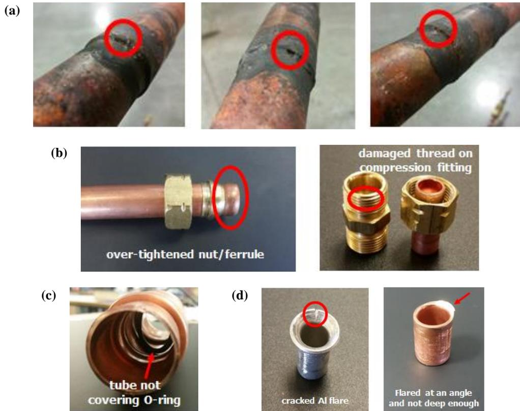
Figure 4: Images of fitting assembly failures: (a) brazed joint, (b) compression fitting, (c) press fitting, and (d) flare fitting.
