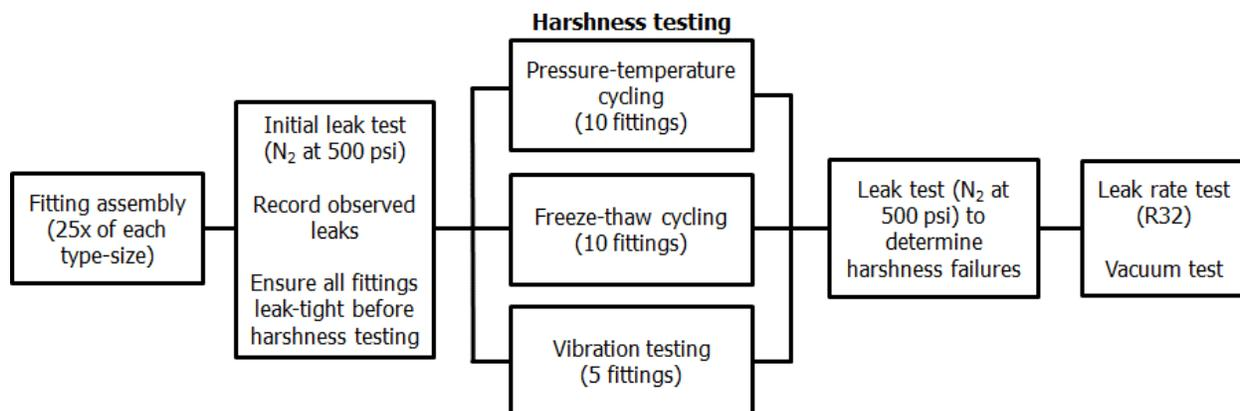
Figure 3: Procedure for evaluation of each fitting in terms of assembly, durability (harshness), and leak rate.
