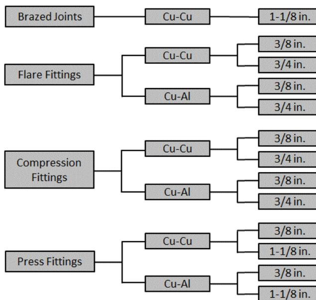
Figure 2: Overview of fitting type-size-material combinations.
