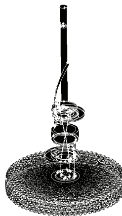
Figure 13: oil supply system model of S-80 compressor Figure 14: mesh of the flow domain for S-80 compressor
