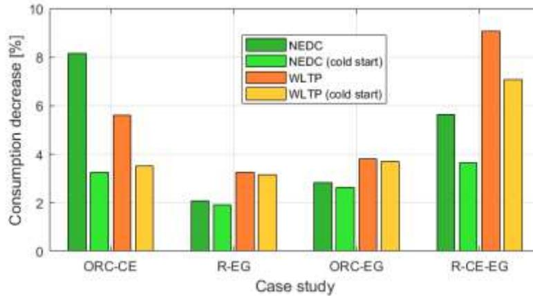
**Figure 8:** Driving cycle performance for 4 different architectures.
