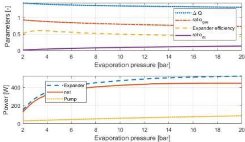
**Figure 3:** Influence of the evaporation pressure on the performance of the system. The performance criteria are shown in the top figure; whereas, the power output of the expander, input power of the pump, and the net power are plotted in the bottom figure.
