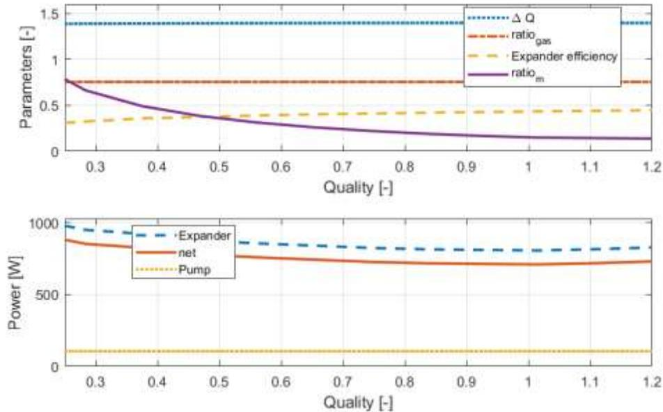
**Figure 4:** Influence of the quality on the performance of the system. The performance criteria are shown in the top figure; whereas, the power output of the expander, input power of the pump, and the net power are plotted in the bottom figure.
