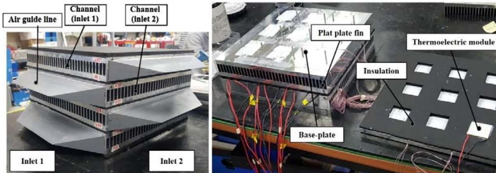
**Figure 4:** Configuration of the inlet side (left) and inside of the thermoelectric air-to-air heat pump unit (right)
