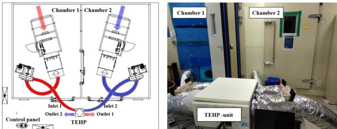
**Figure 5:** Schematic diagram of the experimental setup (left) and a photograph of the thermoelectric heat pump unit (right)
