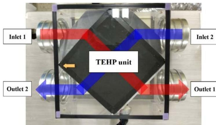
**Figure 3:** Configuration of a cross-flow thermoelectric air-to-air heat pump unit
