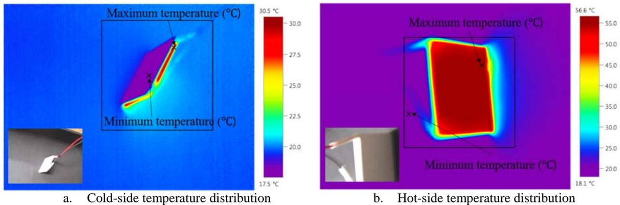
**Figure 1:** Temperature distribution on each side of the thermoelectric module
