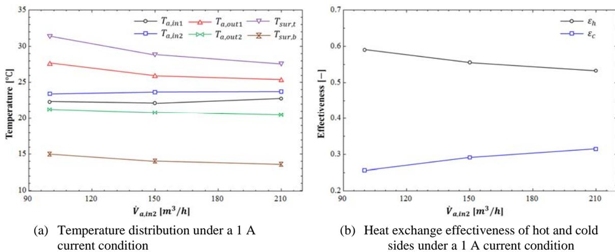
Figure 7: Influence of volume flow rate on the thermoelectric heat pump unit
