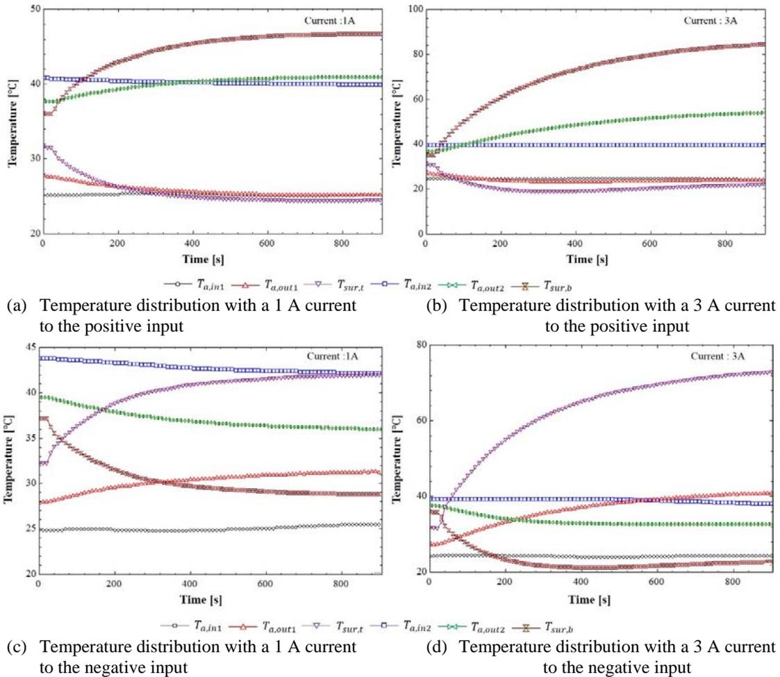
**Figure 8:** Performance of the thermoelectric heat pump unit over time
