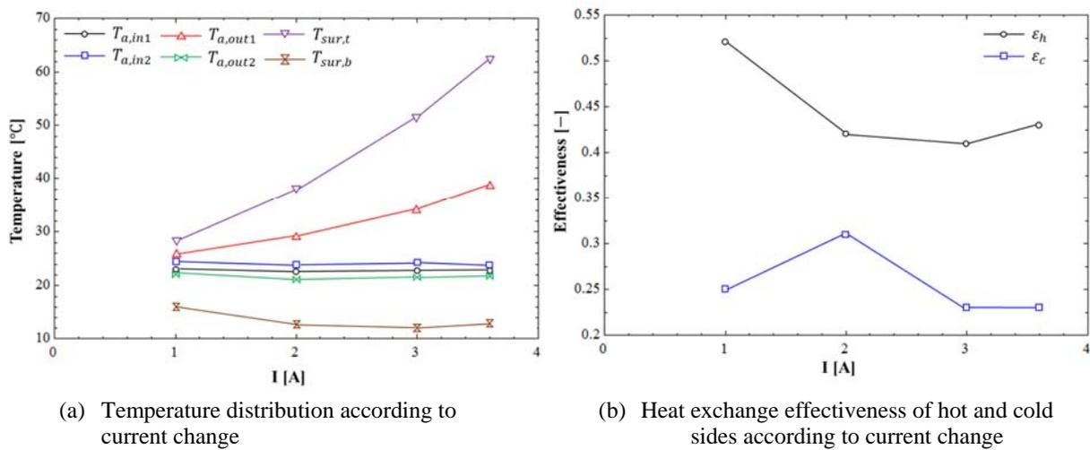
Figure 6: Influence of current on the thermoelectric heat pump unit
