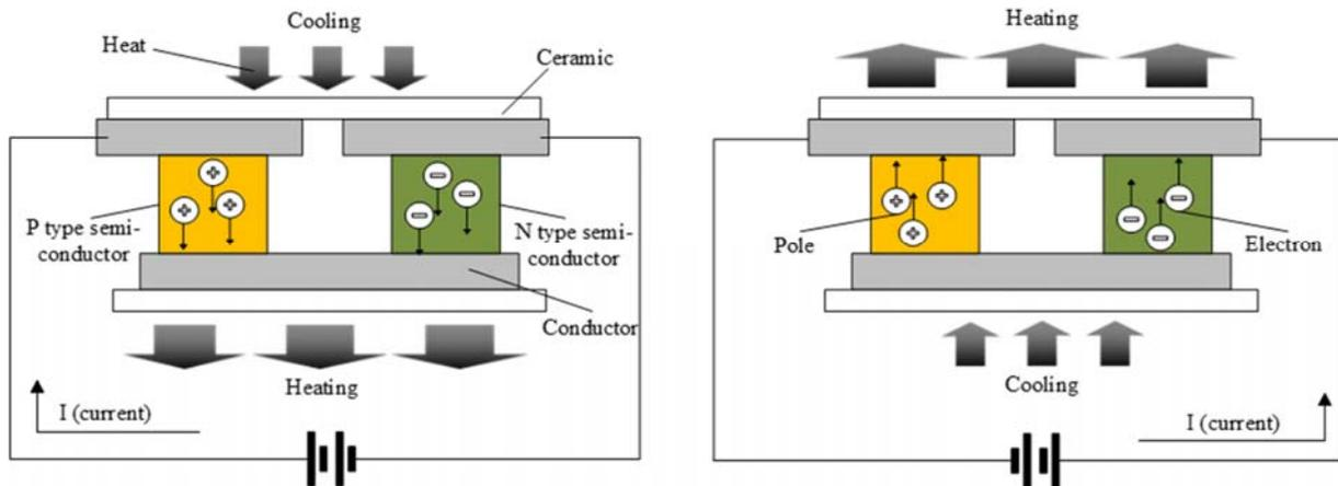
**Figure 2:** Schematic of the thermoelectric element and the Peltier effect
