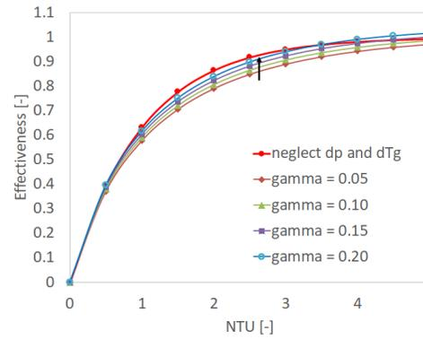
Fig. 12  $\epsilon$  for counter-flow evaporator ( $C_{ratio} = 0.5$ )
