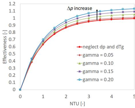
Fig. 9  $\epsilon$  for parallel-flow evaporator ( $C_{ratio} = 0.02$ )
