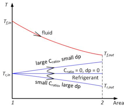
Fig. 13 Temp. profile for a parallel-flow evaporator
