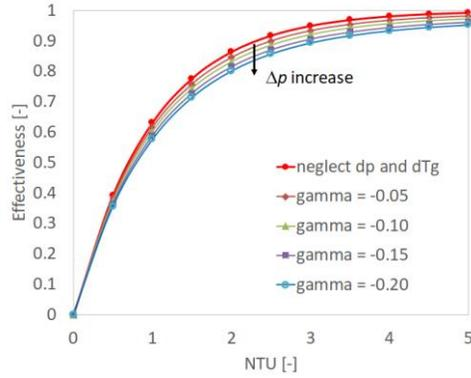
Fig. 8  $\epsilon$  for counter-flow condenser ( $C_{ratio} = 0.02$ )
