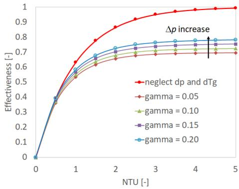
Fig. 11  $\epsilon$  for parallel-flow evaporator ( $C_{ratio} = 0.5$ )
