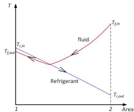
Fig. 14 Temp. crossing in a counter-flow evaporator
