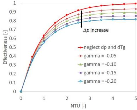
Fig. 7  $\epsilon$  for parallel-flow condenser ( $C_{ratio} = 0.02$ )
