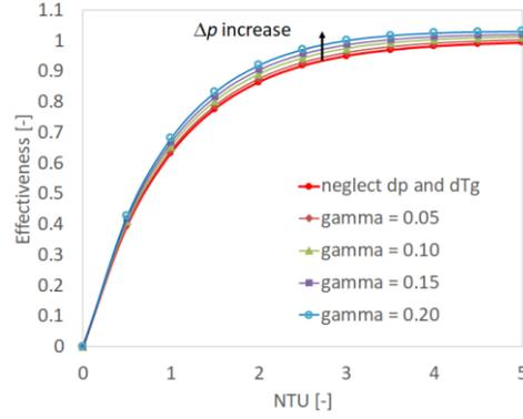
Fig. 10  $\epsilon$  for counter-flow evaporator ( $C_{ratio} = 0.02$ )
