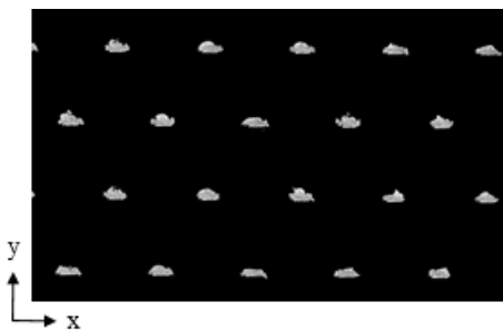
Figure 10: CT scan of fins at minimum diameter
