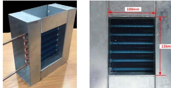
(a) test sample structure rig (b) size of heat exchanger in test sample
