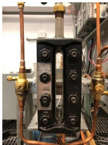
**Figure 5:** Photo of nozzle visualization sight glass
