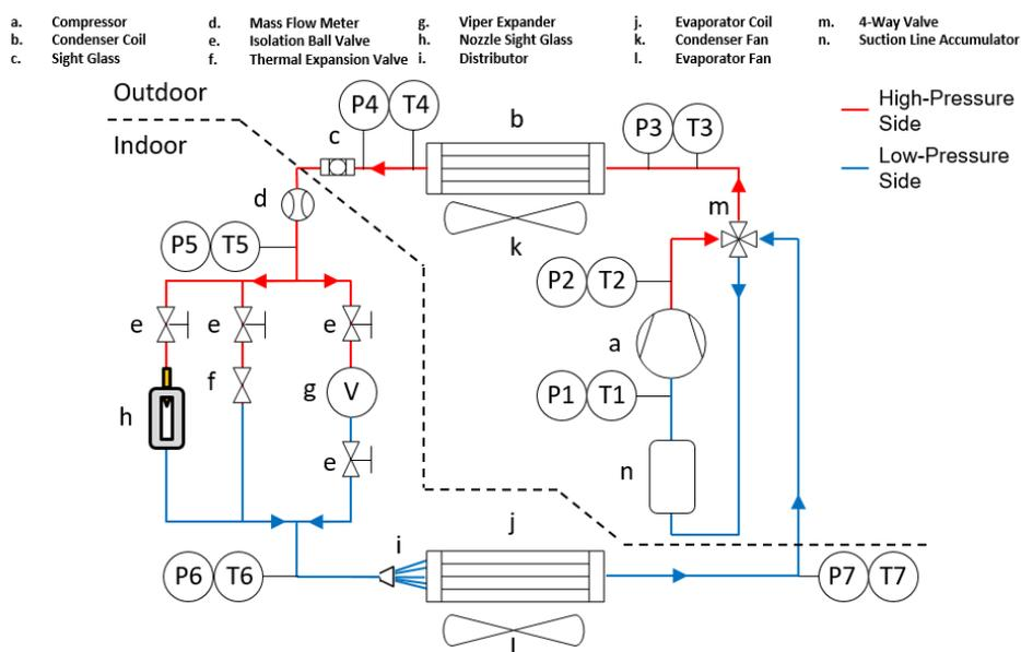
**Figure 6:** 5-Ton heat pump and psychrometric chamber schematic
