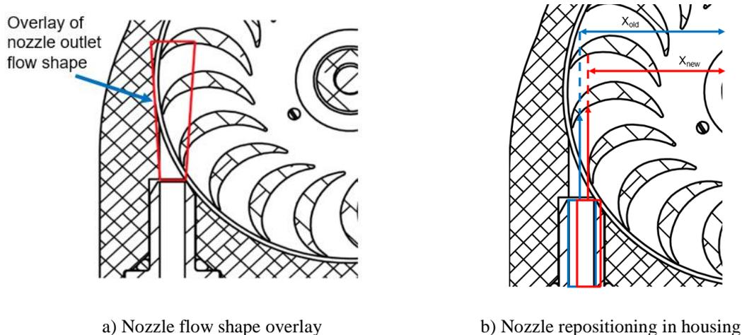
**Figure 8:** Flow geometry overlay on turbine drawing
