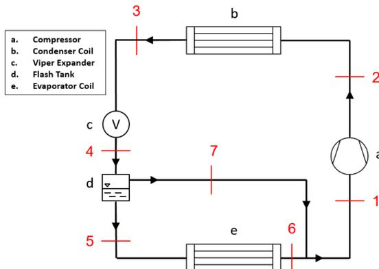
Figure 1: Schematic of expander heat pump cycle
