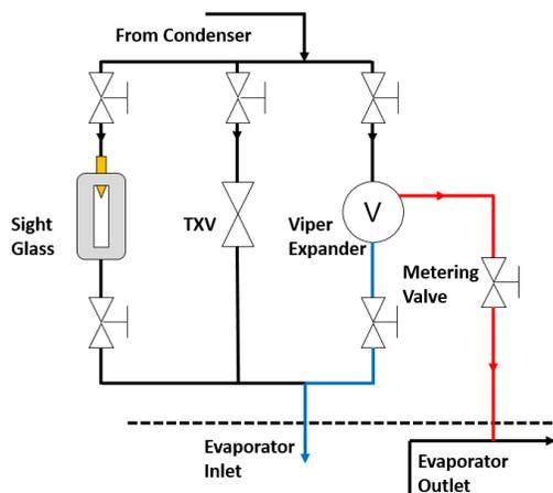
**Figure 4:** Schematic of expansion circuit
