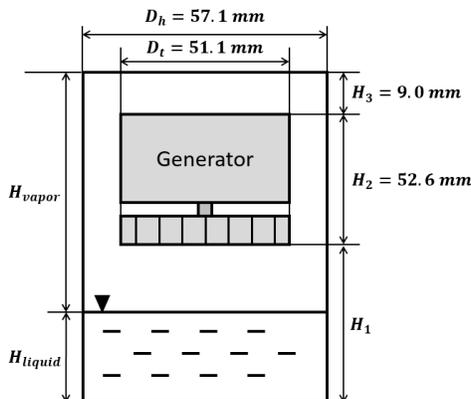
Figure 3: Dimensions of the new expander housing
