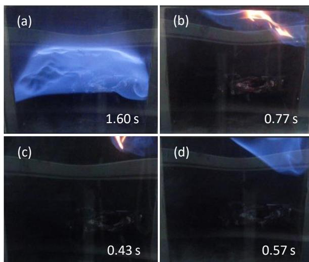
**Figure 5:** Lighter flame insertion results for (a) R-32: 16%, (b) R-1234yf: 8%, (c) R-1234ze: 7.5%, and (d) R-452B: 13%. The largest flames are shown.
