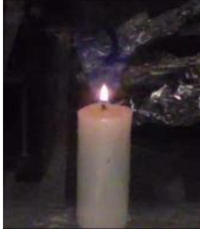
**Figure 6:** From lower leak testing, the candle extinguishes at 4.7% R-32. A blue localized flame is visible. were observed in upper leak candle testing. There was no effect of candle location in the small box.
