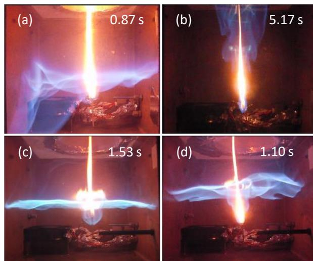
**Figure 4:** Safety match tests: (a) R-32: 17% (LFL = 14.4%), (b) R-1234yf: 7.2% (LFL = 6.2%), (c) R-1234ze: 9.8% (LFL = 6.5%), and (d) R-452B: 15.5% (LFL = 11.9%).
