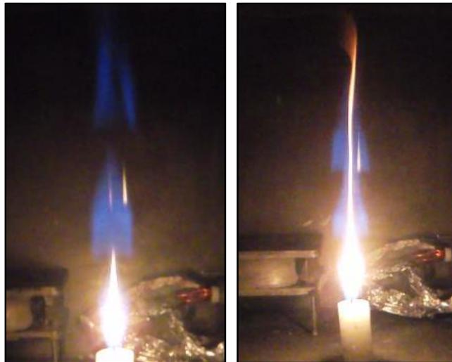
**Figure 7:** Candle tests in R-1234yf: (a) Upper leak with approximately 4% R-1234yf; (b) Lower leak with approximately 3% R-1234yf.
