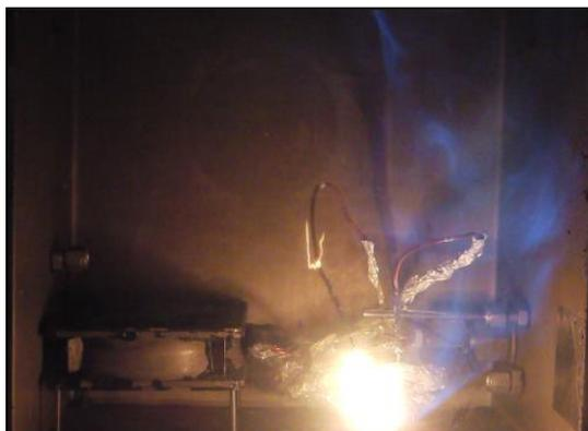
**Figure 2:** Hot wire in R-32 for the diffusion method. The flammability limit is estimated at 3.8% concentration.
