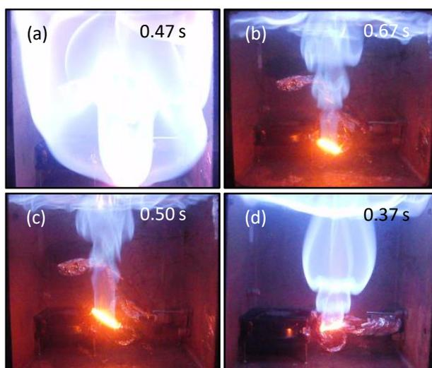
**Figure 3:** Deflagrations seen from slow voltage increase of hot wire in stoichiometric mixtures: (a) R-32; (b) R-1234yf; (c) R-1234ze; and (d) R-452b. Images taken when the propagating flames hit sides of the walls.
