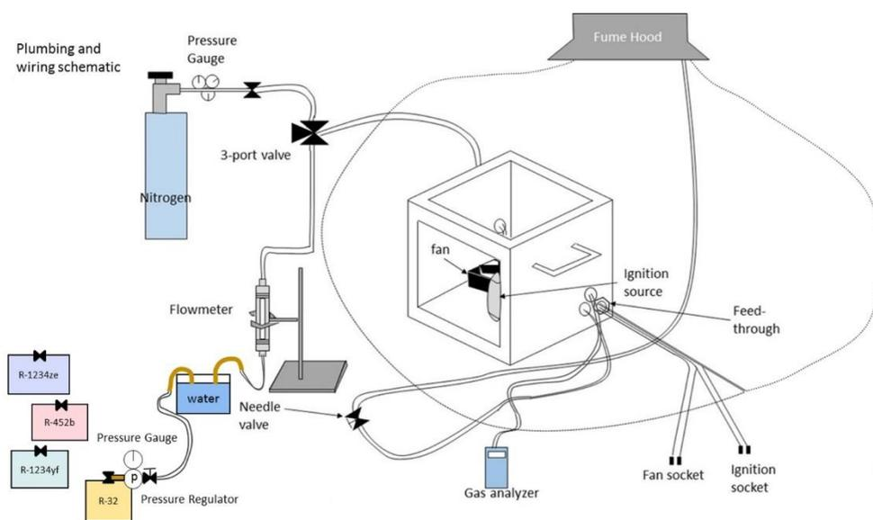
Figure 1: Test Schematic.
