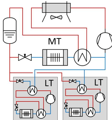
Figure 7. R515A/ R1234yf Cascade Refrigeration System
