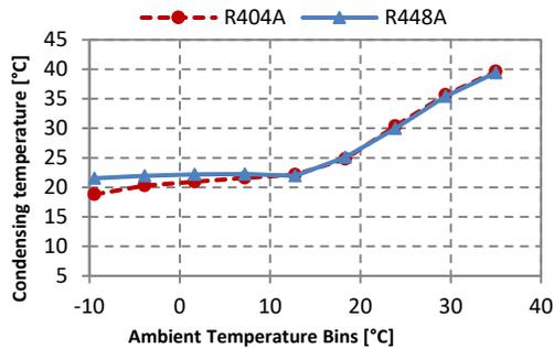
Figure 2. Condensing temperature as a function of the ambient temperature
