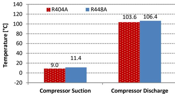
Figure 4. Compressor temperatures at 35°C ambient temperature bin
