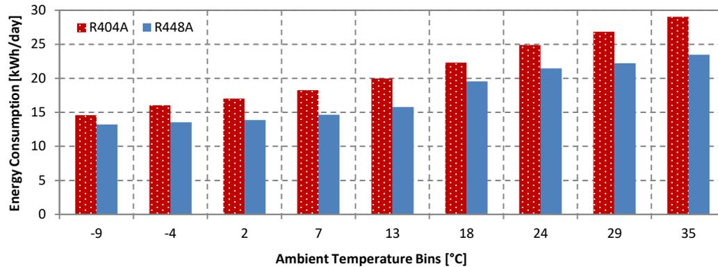
Figure 6. Total system energy consumption as a function of the ambient temperature
