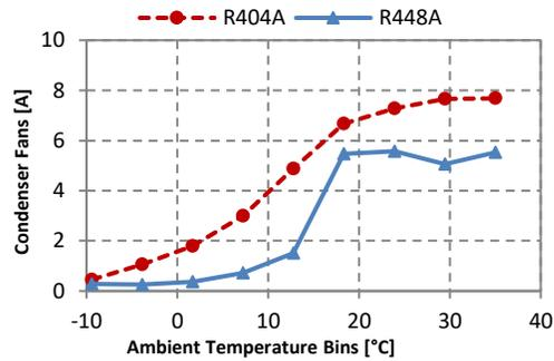
Figure 3. Condenser fan power as a function of the ambient temperature
