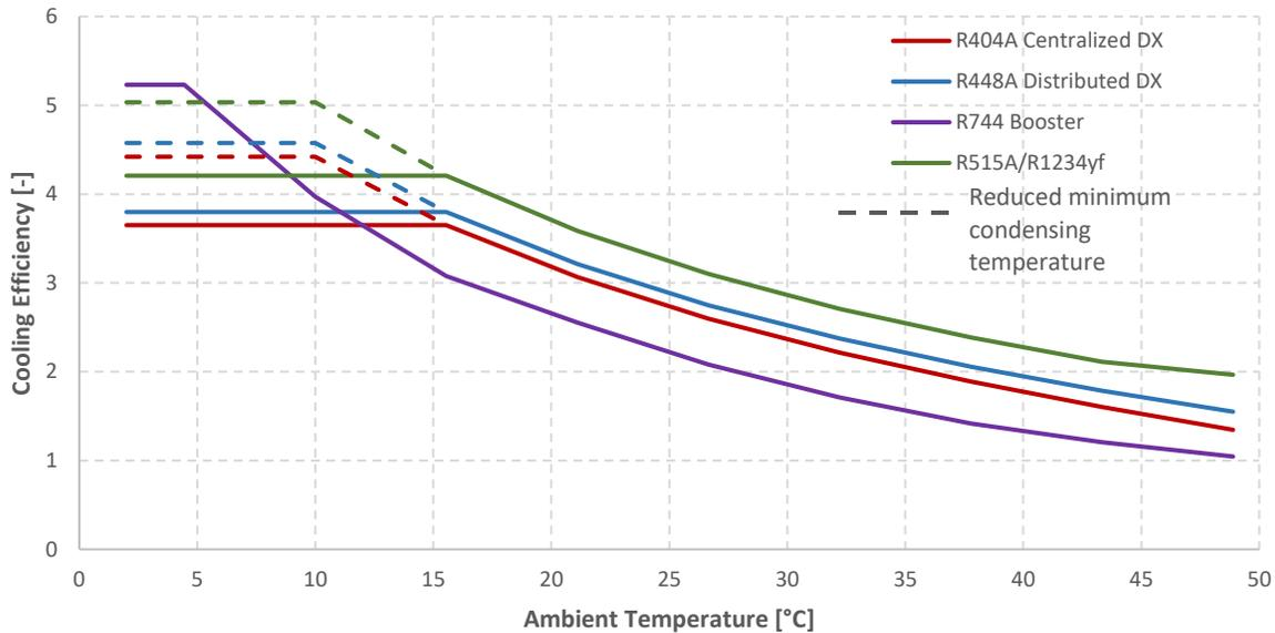
Figure 8. Cooling efficiency of supermarket refrigeration systems at different ambient temperatures
