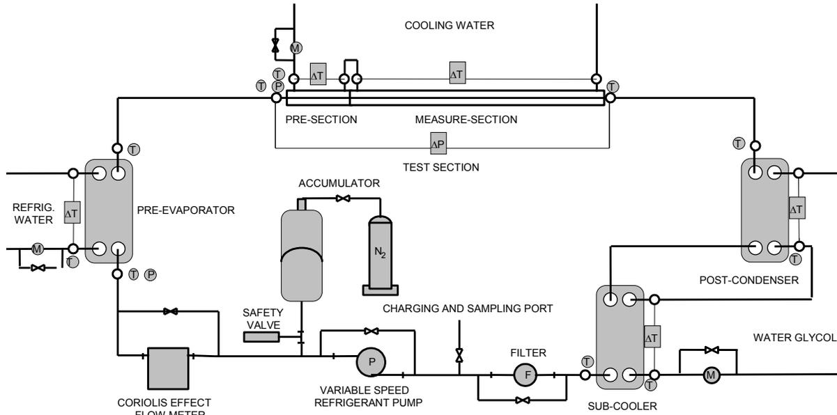
**Figure 1:** Schematic view of the experimental test rig.
