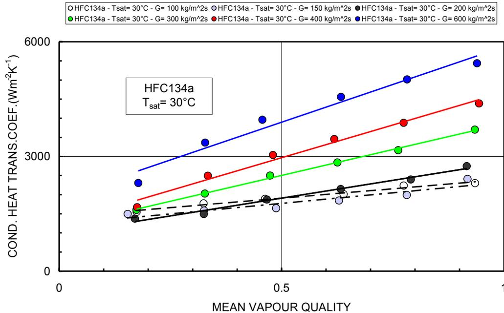
**Figure 2a:** Condensation heat transfer coefficient vs. mean vapour quality and mass flux at  $30^\circ\text{C}$  for HFC134a.
