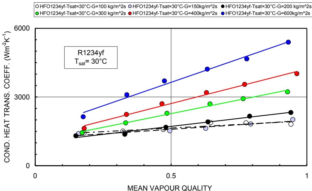
**Figure 2b:** Condensation heat transfer coefficient vs. mean vapour quality and mass flux at  $30^\circ\text{C}$  for HFO1234yf.
