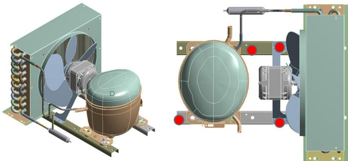
**Figure 1:** Components used in numeric model on left. Fixation point used as boundary condition on right.
