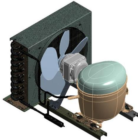
**Figure 2:** Detail optimized mesh. Shell elements used to represent most elements.
