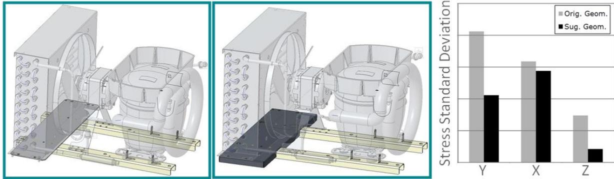
**Figure 9:** Original geometry on left. Proposed geometry on center and stress reduction on right.
