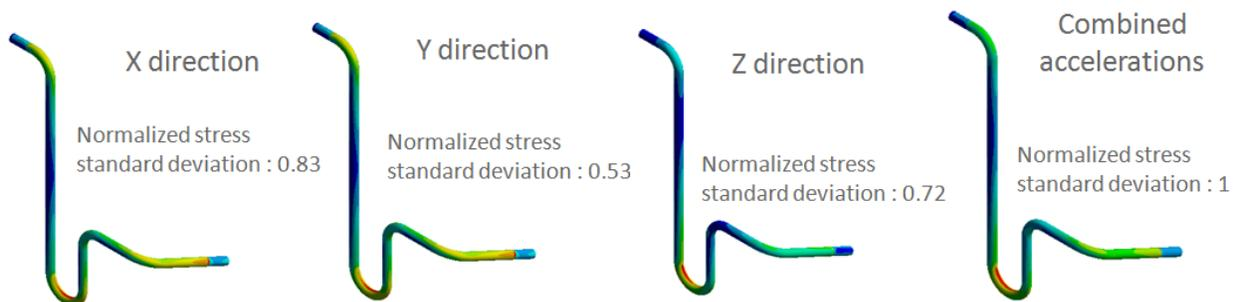
**Figure 4:** Equivalent stress comparison between different accelerations spectrum and directions.
