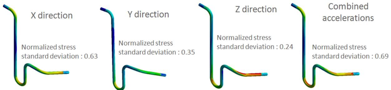
**Figure 10 – Suggested geometry equivalent stress**
