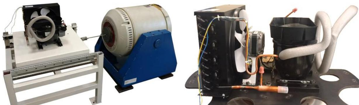
**Figure 6:** Experimental setup. On left a test rig with accelerations on Z direction. On right attest rig with accelerations on Y direction
