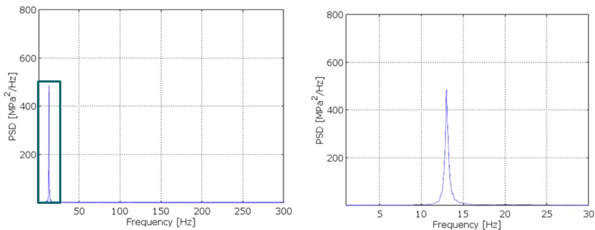
**Figure 8:** Strain gage time series power spectrum density. Detail on lower frequency on left image.
