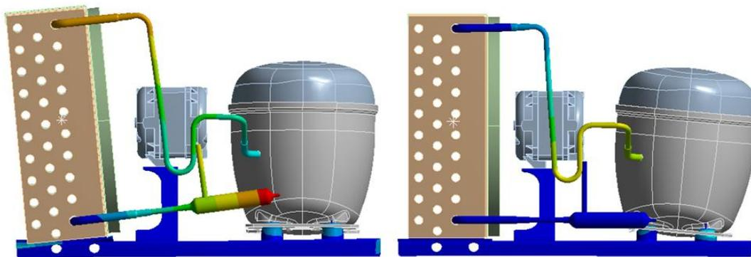
**Figure 5:** Two most relevant modes. On left the mode related to the condensing unit fixation, on right the mode related to the compressor fixation.
