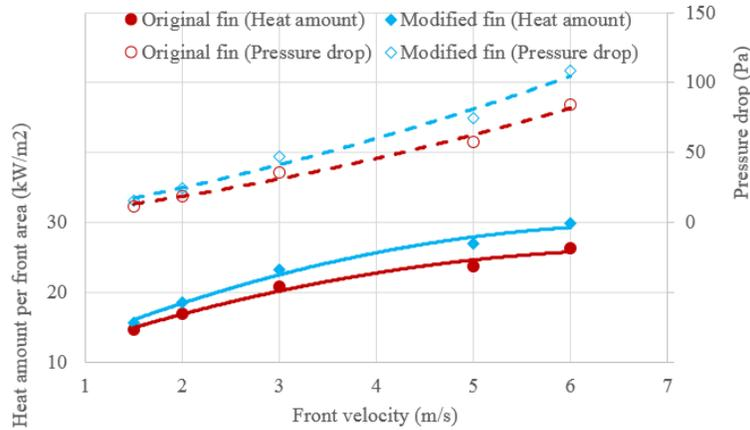
**Figure 6:** Experimental results of modified fin performance
