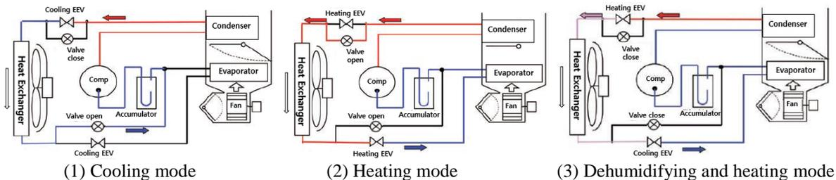
Figure 3: Automotive heat pump cycle
