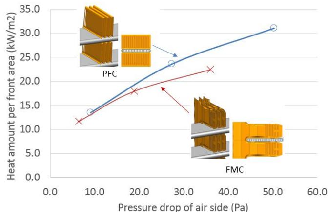
**Figure 4:** Comparison of performance between PFC and FMC
