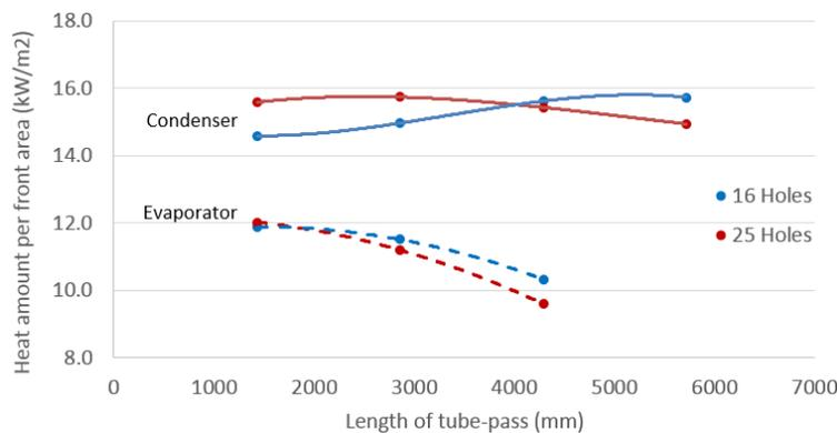
**Figure 7:** Influence on performance of hole size and tube-pass length
