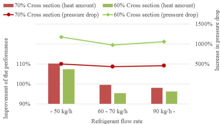
Figure 11: Improvement of refrigerant distribution by cross section of header
