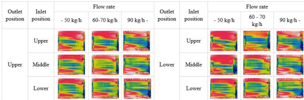
(a) Image of refrigerant distribution by IR camera (Evaporation)
