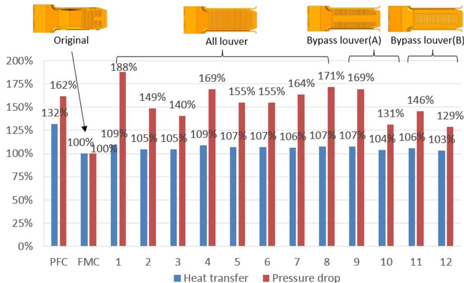
**Figure 5:** Results of the analysis for fin shape (STAR-CCM+11.02.009)
