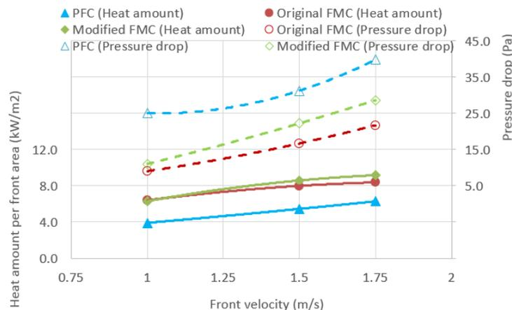
(b) Comparison of performance and pressure drop (Evaporation)
