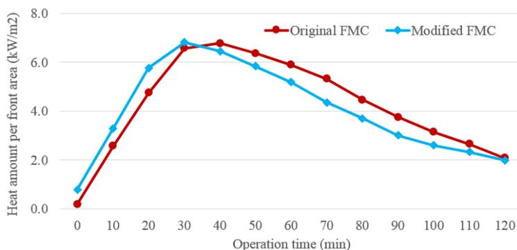
**Figure 13:** Comparison of frost performance (FMC vs. Modified FMC)
