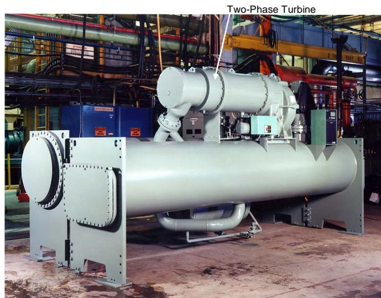
**Figure 4:** Commercial Chiller with Two-Phase Impulse Turbine Installed
