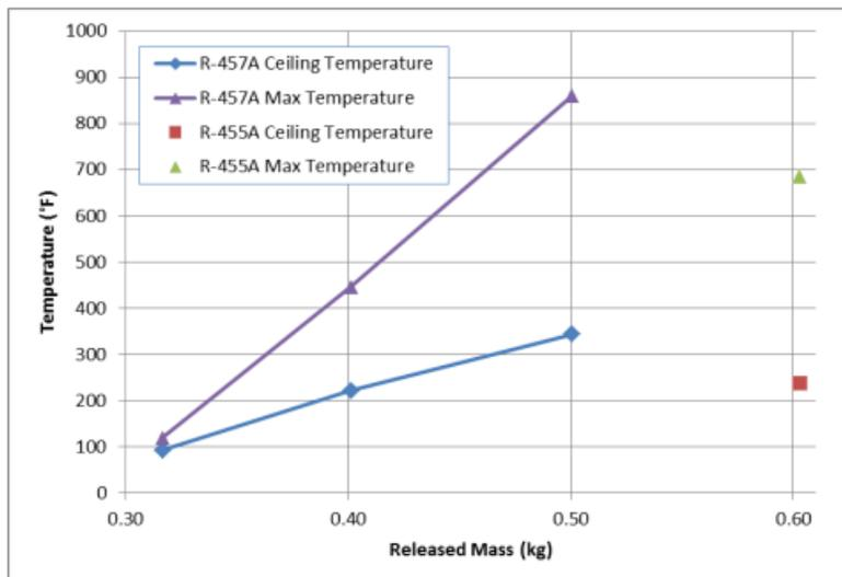
Figure 7: Measured temperatures in reach-in cooler testing (Gandhi et al, 2017)
