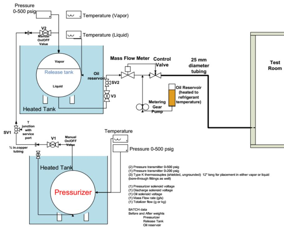
Figure 1: Schematic of the refrigerant release mechanism setup (Gandhi et al, 2017)
