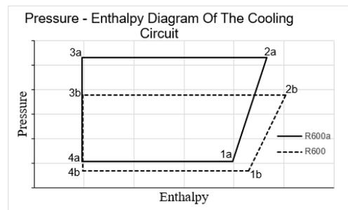
Figure 5 pressure - enthalpy diagram of the cooling circuit (R600a and R600)
