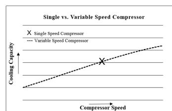
**Figure 2** Comparison of the cooling capacity of single and variable speed compressors as a function of compressor speed.
