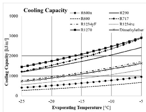
**Figure 4** Volumetric cooling capacity of different refrigerants
