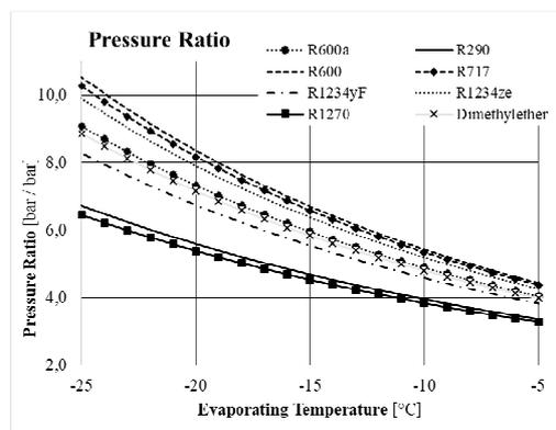
**Figure 3** Pressure ratio of different refrigerants
