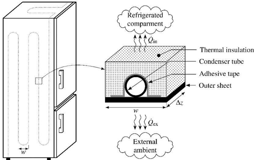
**Figure 1:** Condenser discretization
