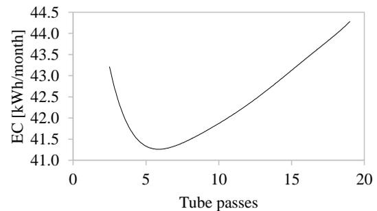
**Figure 14:** Energy consumption as a function of the number of tube passes
