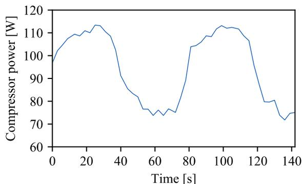
**Figure 11:** Compressor power soon after compressor start-up
