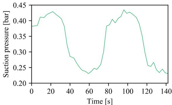
**Figure 9:** Suction pressure soon after compressor start-up
