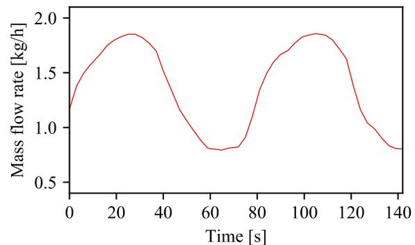
**Figure 10:** Mass flow rate soon after compressor start-up
