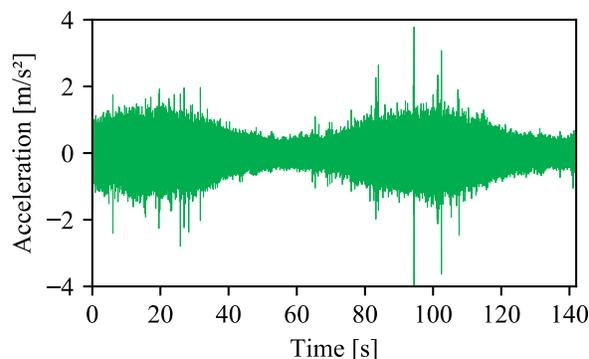
**Figure 12:** Accelerometer readings soon after compressor start-up
