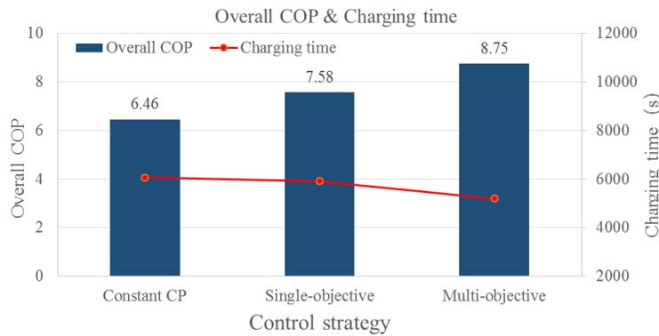
Figure 5: Comparison of overall COPs and charging time
