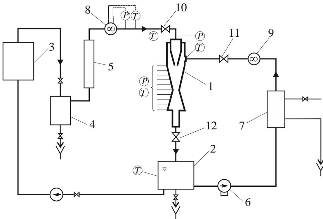
**Figure 4:** Schematic diagram of the experimental stand: 1 – low pressure steam-water injector, 2 – water tank, 3 – steam generator, 4 – steam separator, 5 – steam superheater, 6 – water pump, 7 – water cooler, 8 – steam flow meter, 9 – water flow meter, 10 – steam pressure control valve, 11 – water flow control valve, 12 – back-pressure control valve.
