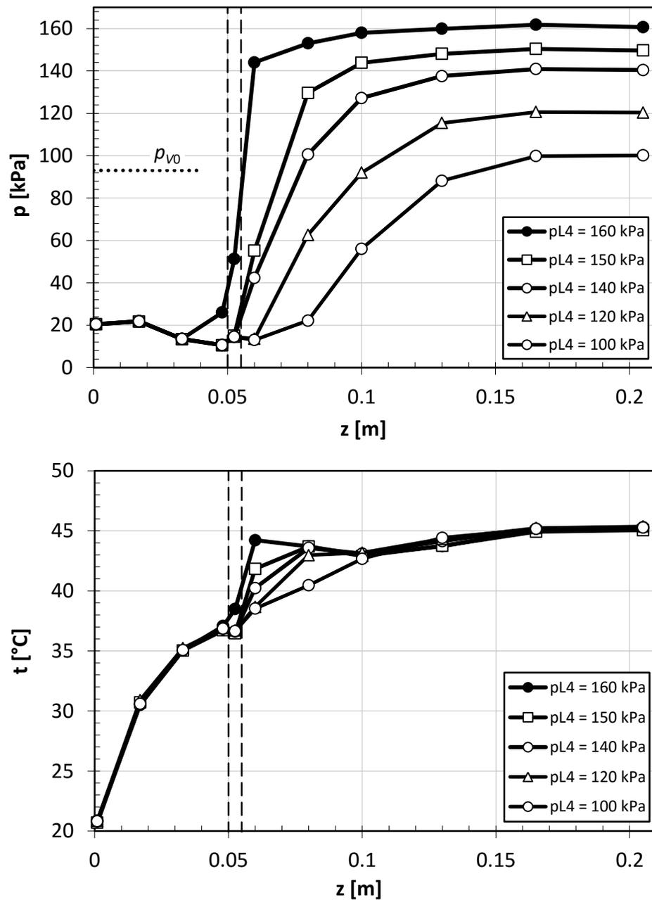
**Figure 5:** Distributions of average pressure  $p$  and temperature  $t$  along the LPSI mixing chamber and diffuser wall measured for constant inlet flow parameters and selected values of back-pressure  $p_{L4}$ . Dashed lines indicate the extent of cylindrical throat. Inlet steam parameters: pressure 93 kPa (shown in pressure diagram as  $p_{v0}$ ), mass flow rate 111 kg/h, superheating 27 °C. Inlet water parameters: temperature 20 °C, mass flow rate 2670 kg/h.
