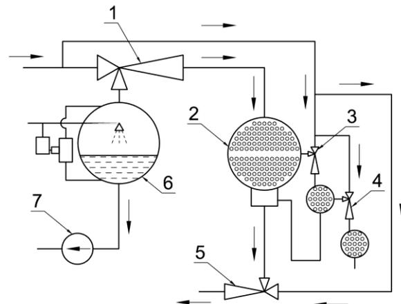
**Figure 2:** Modified steam ejection refrigeration system with two-phase injector as a liquid pump: 1 – motive ejector; 2 – condenser; 3 – ejector vacuum pump of 1<sup>st</sup> step; 4 – ejector vacuum pump of 2<sup>nd</sup> step; 5 – steam-water injector; 6 – evaporator; 7 – cold water pump.
