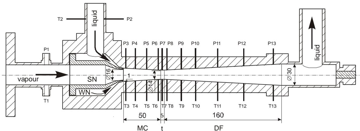
**Figure 3:** Schematic and principal dimensions of the investigated low pressure steam–water injector: SN – steam nozzle, WN – water nozzle, MC – mixing chamber, DF – diffuser,  $t$  – throat, T1 - T13 – temperature measurement, P1 - P13 – pressure measurement.
