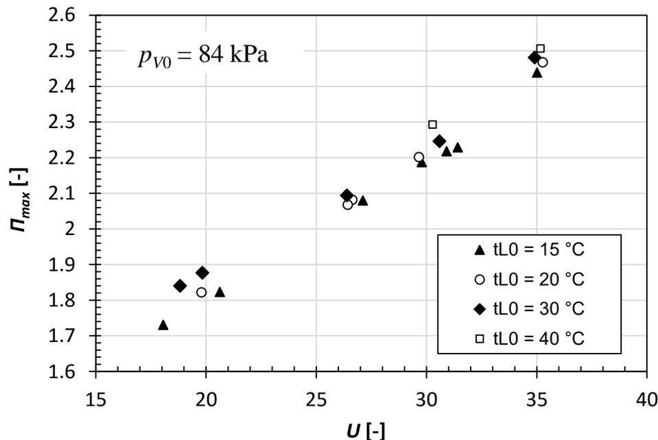
**Figure 7:** Compression ratio  $\Pi$  as a function of entrainment ratio  $U$  calculated for the LPSI driven by a steam at pressure  $p_{V0} = 84$  kPa, flow rate 100 kg/h and superheating 26 °C. Inlet water temperature  $t_{L0}$  was in the range 15 - 40 °C.
