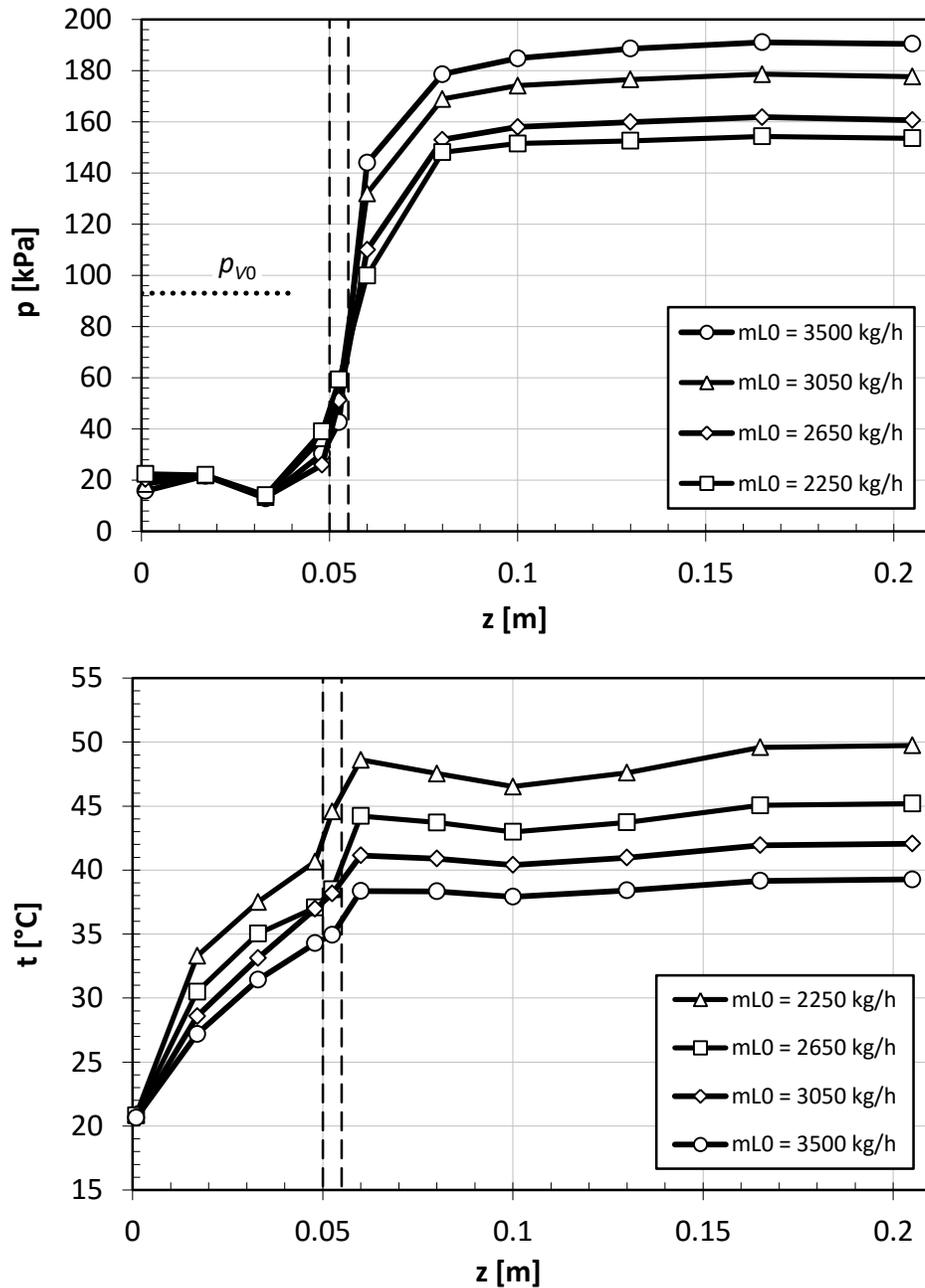
**Figure 6:** Distributions of average pressure  $p$  and temperature  $t$  along the LPSI mixing chamber and diffuser wall measured for three selected water flow rates  $\dot{m}_{L0}$  at near-maximum back-pressure. Dashed line indicates the extent of cylindrical throat. Inlet steam parameters: pressure 93 kPa (shown in pressure diagram as  $p_{v0}$ ), mass flow rate 111 kg/h, superheating 26 °C. Inlet water temperature 20 °C.
