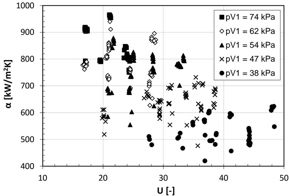
**Figure 8:** Average heat transfer coefficient  $\alpha$  calculated from pressure and temperature distributions in the LPSI mixing chamber. The points are grouped by mixing chamber inlet pressure  $p_{V1}$ .
