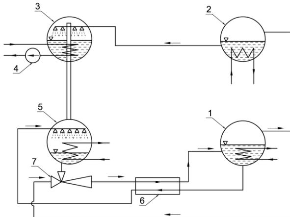
**Figure 1:** Modified absorption LiBr refrigeration system with two-phase injector as a liquid pump: 1 – steam generator; 2 – condenser; 3 – evaporator; 4 – cold water pump; 5 – absorber; 6 – internal heat exchanger; 7 – steam-water injector.
