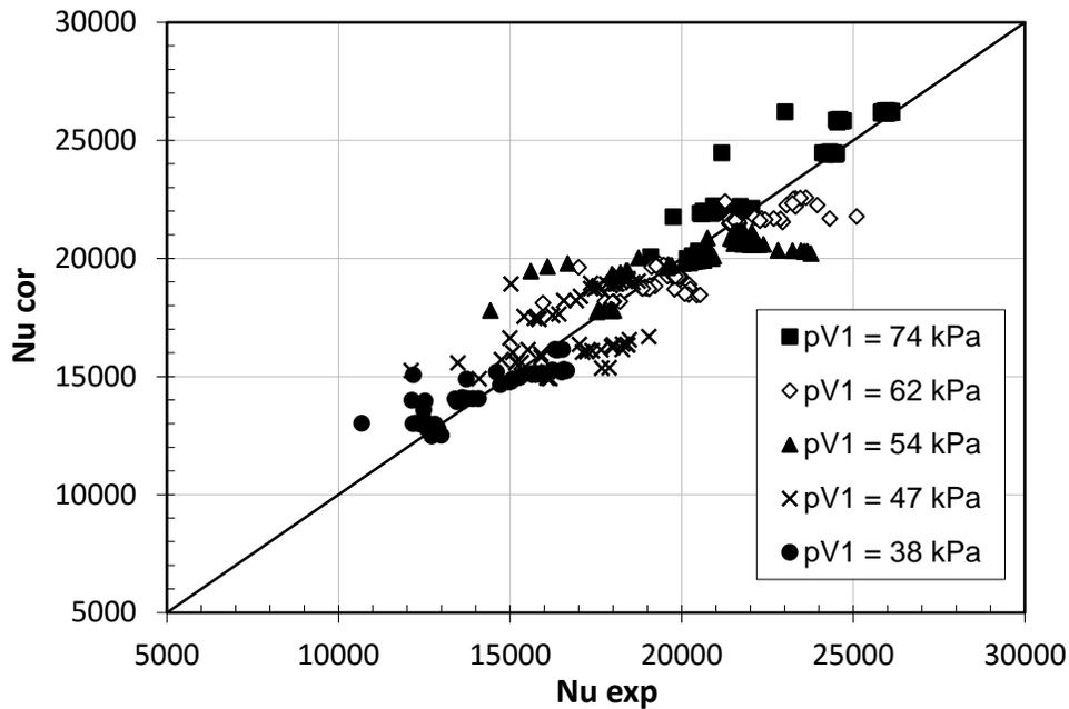
**Figure 9:** Correlated (6) vs experimental average heat transfer coefficient  $\alpha$  for LPSI mixing chamber. The points are grouped by mixing chamber inlet pressure  $p_{V1}$ .
