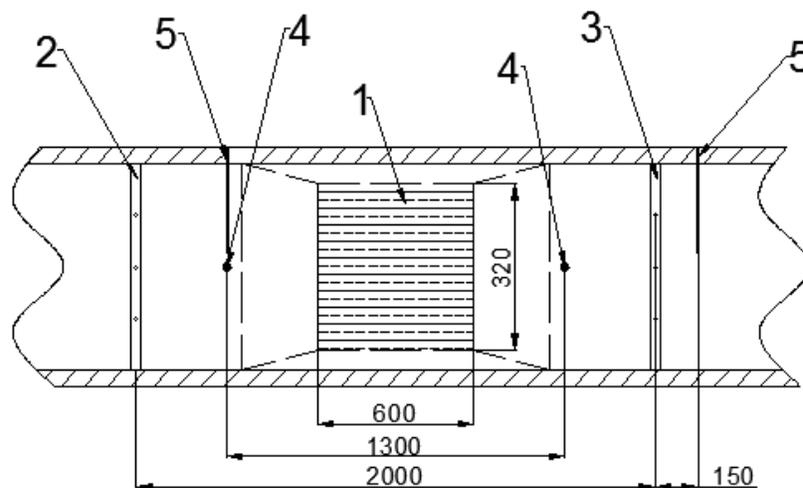
**Figure 3.** Schematic of the test section: 1- tested packed bed; 2- thermocouples net at the bed inlet; 3 - thermocouples net at the bed outlet; 4- pressure gauges; 5- air moisture sensors
