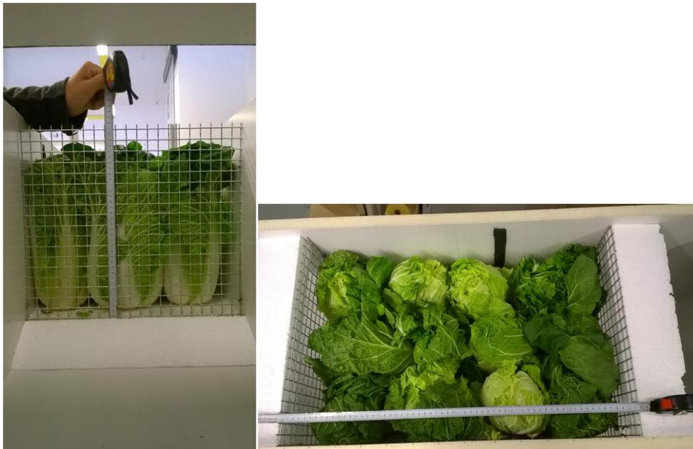
**Figure 4.** The packed Bed of Chinese cabbage prepared for insertion to the test channel
