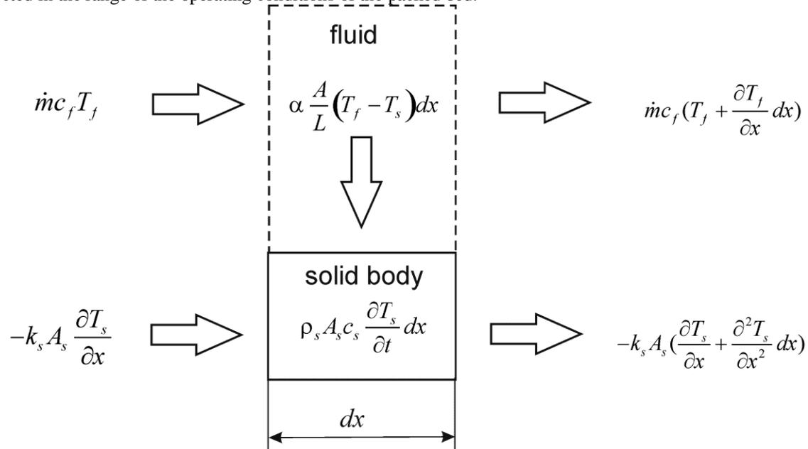
**Figure 1.** Energy balance for fluid (f) and solid body (s) for heater exchanger element
