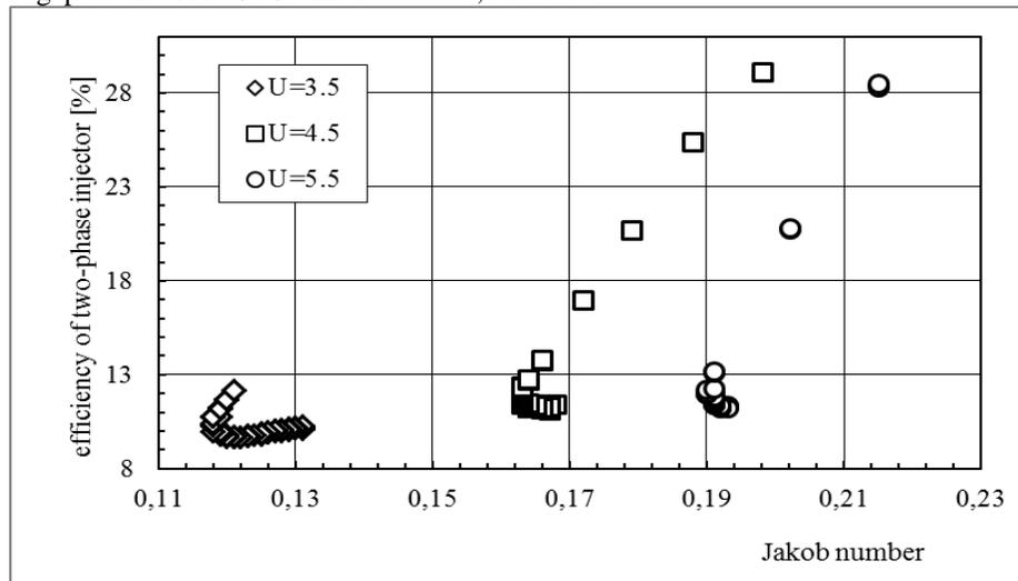
**Figure 5.** Relationship between total injector efficiency  $\eta_e$  versus Jakob number  $Ja$ .
