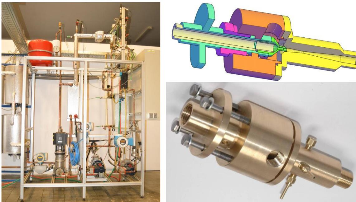
**Figure 4.** Photo of testing stand (left) and tested two-phase injector (right) equipped with the motive nozzle of the throat diameter 1.5 mm; the diameter of the mixing chamber 2.2 mm.
