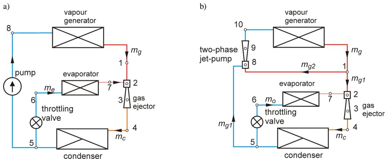
**Figure 1.** Diagrams of ejection refrigeration systems:
