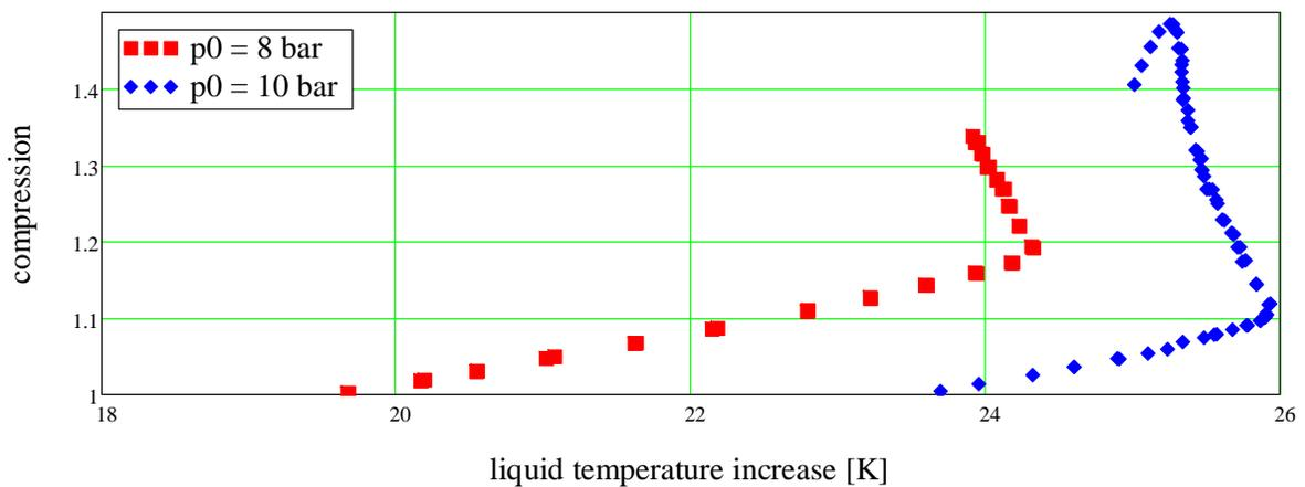
**Figure 8.** Compression ratio versus liquid phase temperature increase for various motive pressures.
