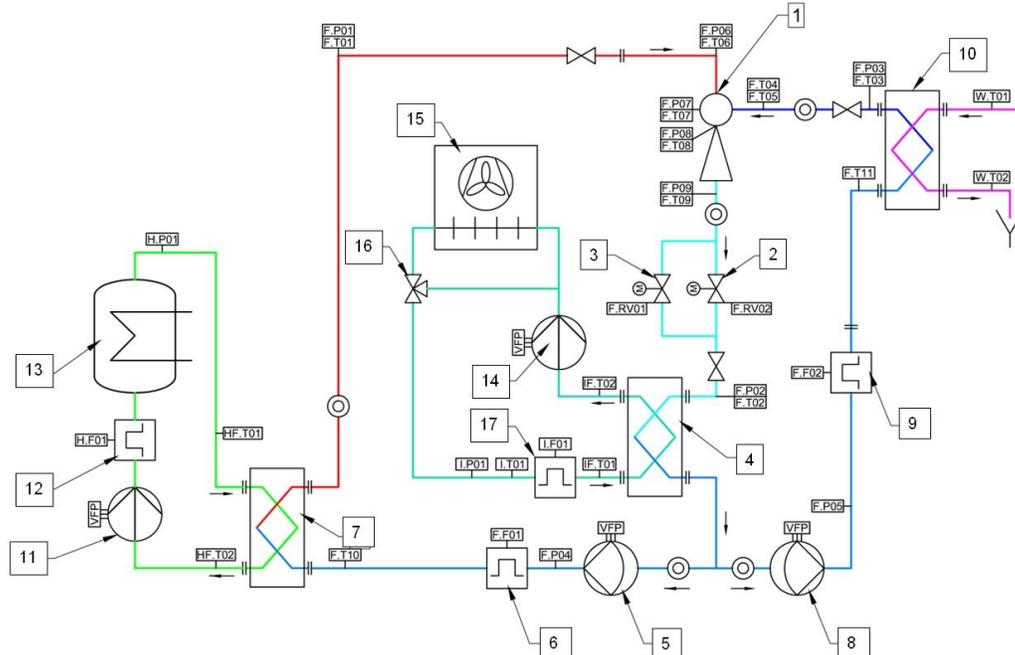
**Figure 3.** Schematic of the testing rig: 1 – tested injector; 2,3 – control valve; 4 – condenser; 5,8 – circulating pump of working fluid; 6,9 – mass flow meter; 7 – vapour generator; 10 – liquid subcooler; 11 – circulating pump of glycol; 12 – mass flow meter; 13 – electric heater; 14 – circulating pump of glycol, 15 – fan cooler; 16 – control valve; 17 – mass flow meter.
