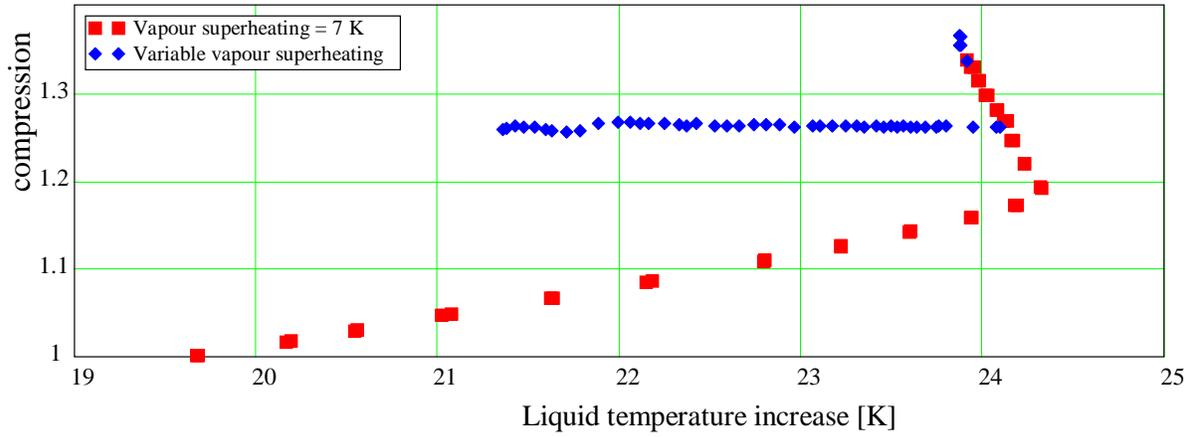
**Figure 9.** Compression ratio versus liquid phase temperature increase for various vapour superheating:
