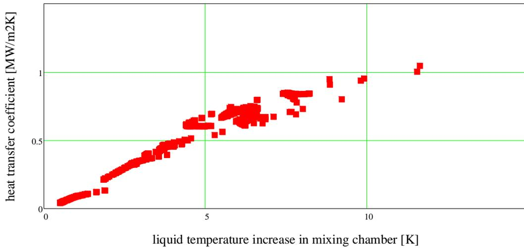
**Figure 7.** Condensation film heat transfer coefficient versus temperature increase of liquid phase.
