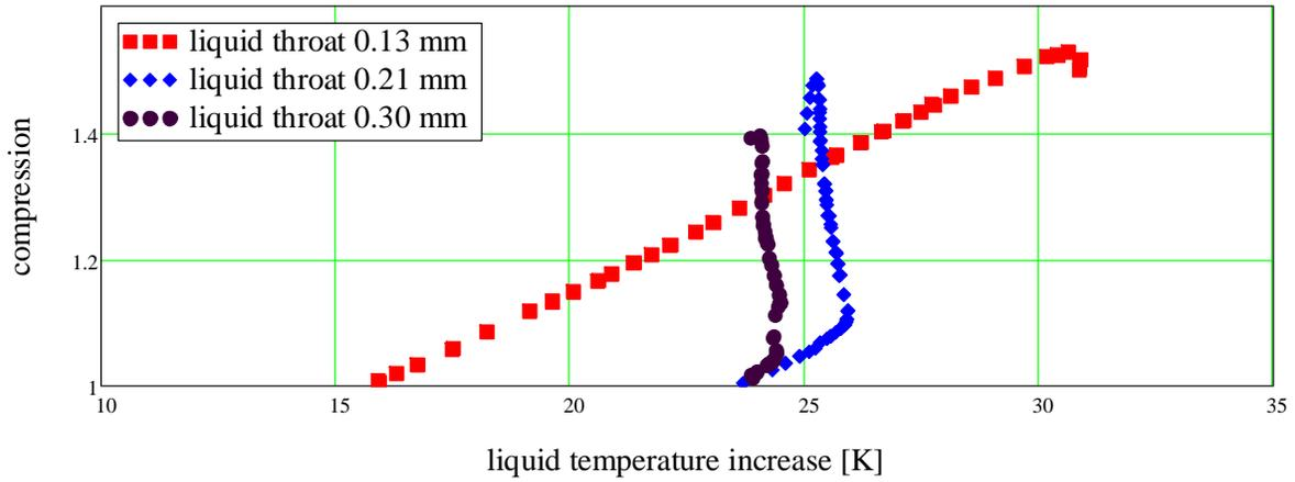
**Figure 6.** Performance characteristics of the injector operations for various liquid nozzle gaps thickness.
