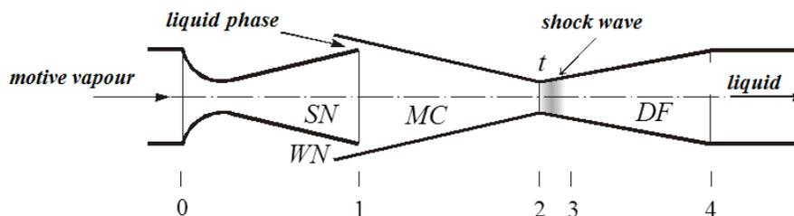
**Figure 2.** Schematic of vapour-liquid injector: SN – motive vapour nozzle, WN – liquid nozzle, MC – mixing chamber, DF – diffuser, t – mixing chamber throat.
