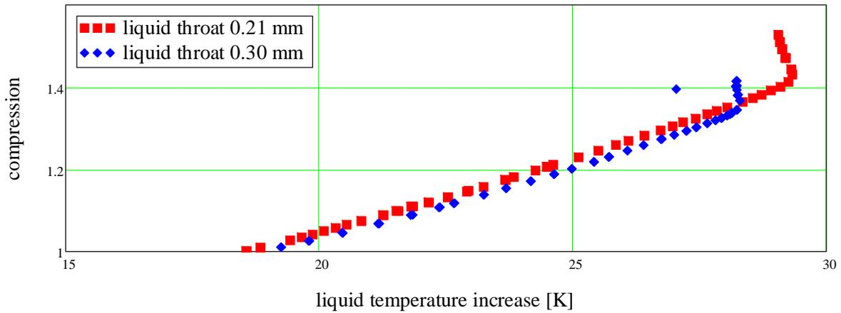
**Figure 11.** Compression ratio versus liquid phase temperature increase for:  $U = 3.5, p_V = 10 \text{ bar}$ .
