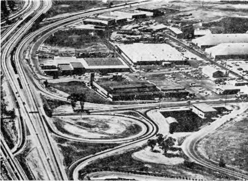
Fig. 5. This is the same area as indicated in Fig. 4, five years later (1959). Many new industries have now located in this interchange area, as close to the expressway facilities as possible. Each of these generate considerable volumes of traffic.
