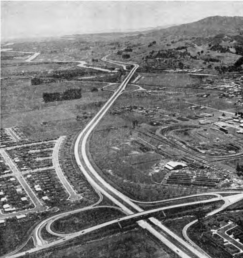
Fig. 8. Several interchange areas on the West Coast. Note the partial interchange in the foreground and how the adjacent residential development is insulated from the interchange ramps and without any direct connections to it. Legal controls and proper design can go a long way toward regulating private land uses in interchange areas in the public interest.
