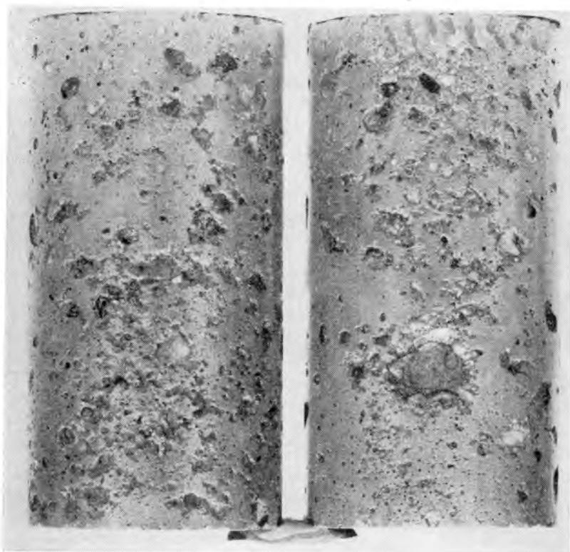
Fig. 2. Pop-outs in three- by six-in. cylinders after 30 cycles of freezing and thawing in water. Concrete contained aggregate graded up to  $\frac{3}{4}$ -in. maximum size w/c 0.51 by weight of cement, 4.2 per cent entrained air. Specimens were fog cured for 14 days followed by 76 days of storage at 50 per cent relative humidity before starting freezing and thawing tests. Pop-outs resulted from soft calcareous siltstones, calcareous cherts, shaly limestones, and ferruginous concretions.
