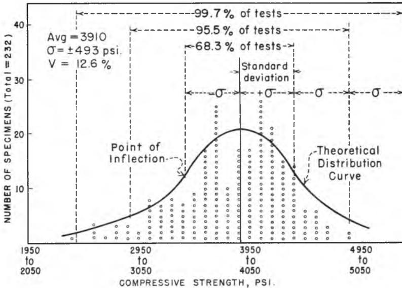
Fig. 13. Typical frequency distribution of compressive strength of six-by 12-in. control cylinders (Angostura Dam, 1948 season).
