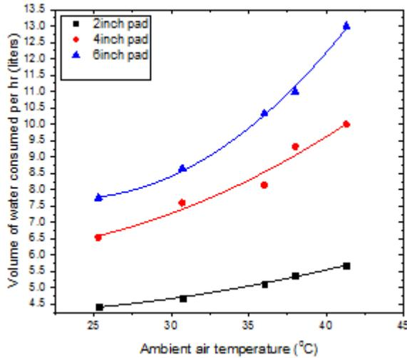
**Figure 7:** Hourly water consumption for each pad thickness at different ambient temperature
