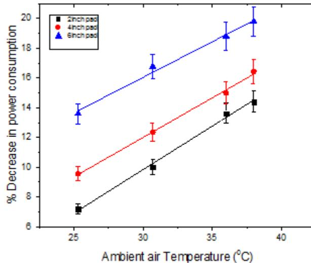
**Figure 5:** Percentage drop in Power consumption at different ambient temperatures
