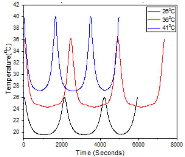
Figure 10: Temperature Profile of the air in the 4inch pad
