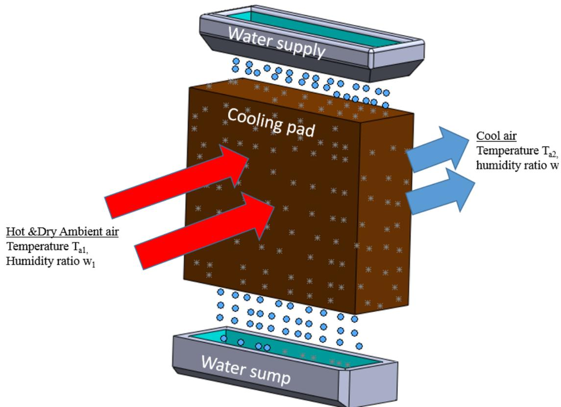
Figure 1: How evaporative cooling works
