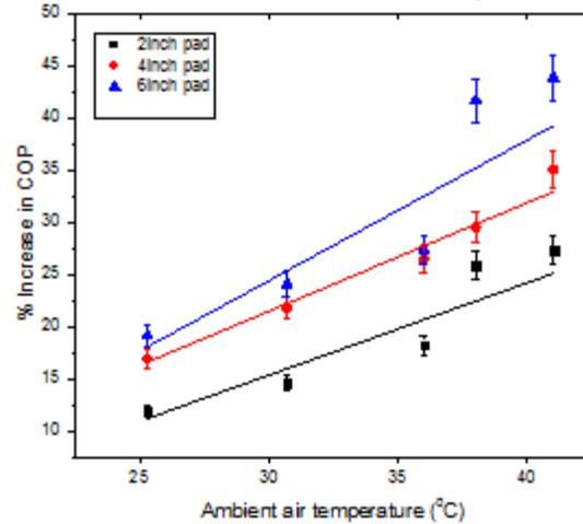
**Figure 4:** Percentage drop in COP at different ambient at different ambient air temperature
