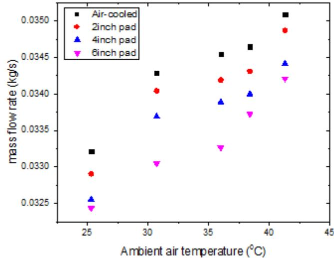
Figure 6: Mass flow-rate of the refrigerant with increase in ambient temperature
