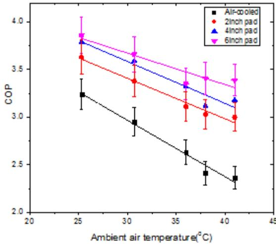
**Figure 3:** COP of the system at different ambient Temperatures
