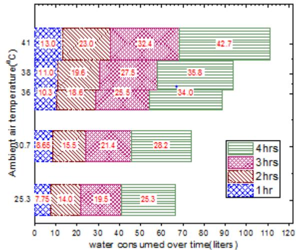
**Figure 8:** Variation of water consumed as operation time increases at different ambient temperature for the 6inch pad
