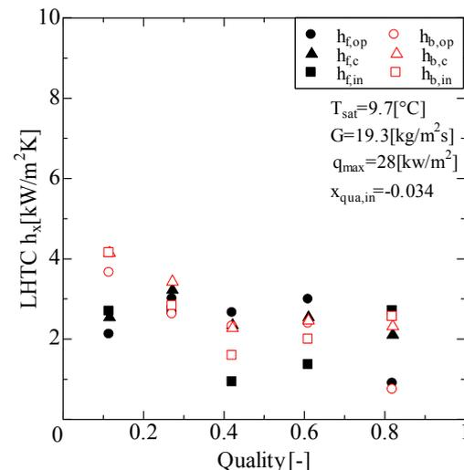
Figure 10: Local heat transfer coefficient of evaporation experiment ( $G = 20$  kg/m<sup>2</sup>s)
