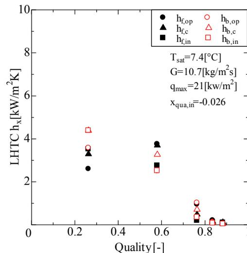
Figure 8: Local heat transfer coefficient of evaporation experiment ( $G = 10$  kg/m<sup>2</sup>s)
