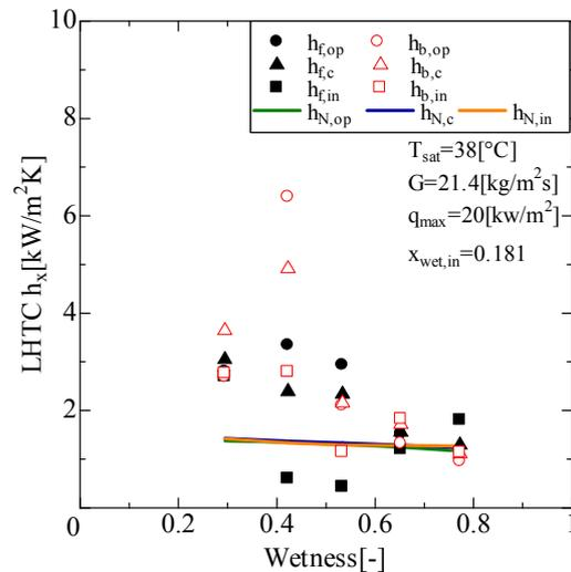
**Figure 6:** Local heat transfer coefficient of condensation experiment ( $G = 20 \text{ kg/m}^2\text{s}$ )
