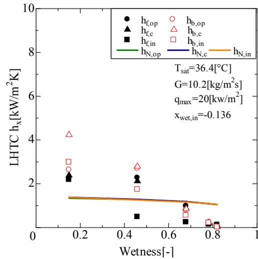
**Figure 4:** Local heat transfer coefficient of condensation experiment ( $G = 10 \text{ kg/m}^2\text{s}$ )
