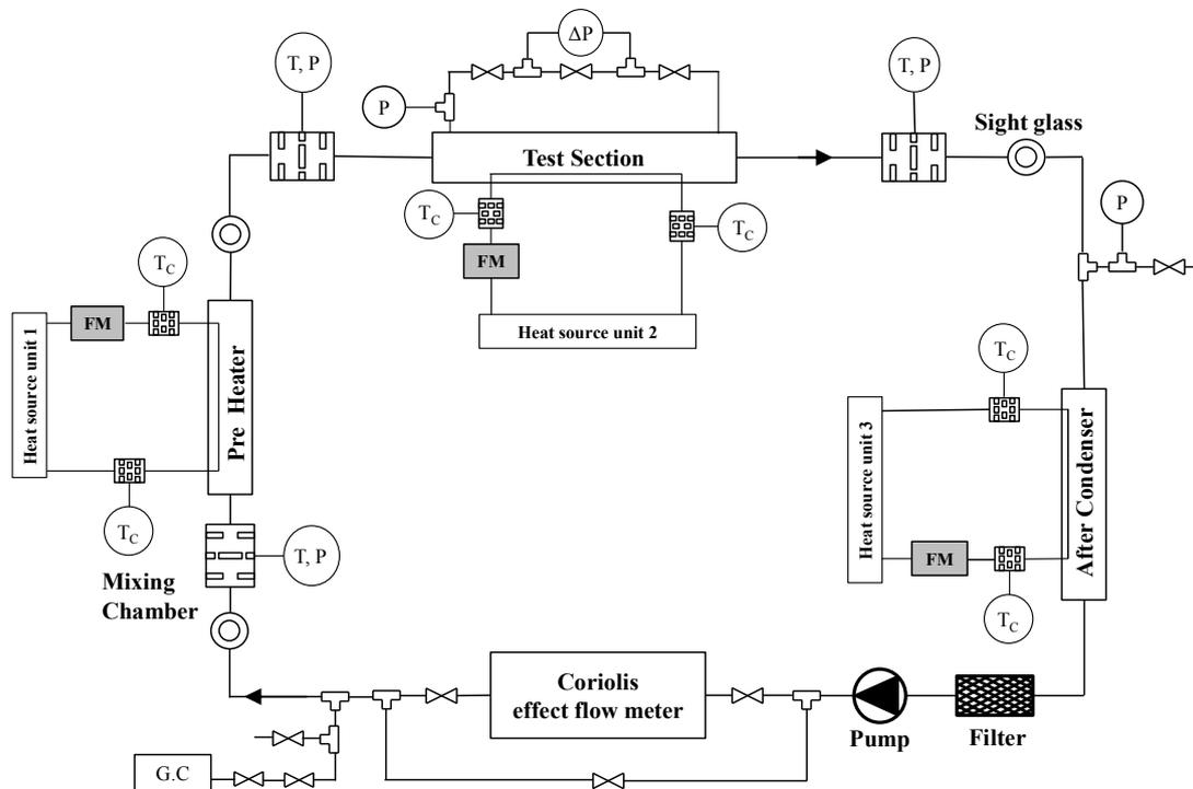
Figure 1: Schematic diagram of refrigerant flow loop
