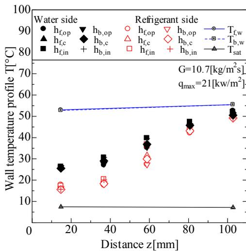
Figure 7: Temperature distribution of wall in evaporation experiment ( $G = 10$  kg/m<sup>2</sup>s)
