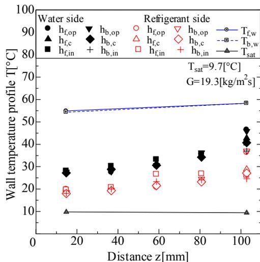
Figure 9: Temperature distribution of wall in evaporation experiment ( $G = 20$  kg/m<sup>2</sup>s)
