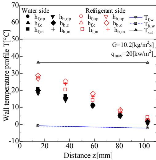
**Figure 3:** Temperature distribution of wall in condensation experiment ( $G = 10 \text{ kg/m}^2\text{s}$ )
