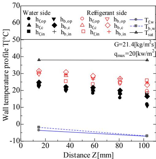
**Figure 5:** Temperature distribution of wall in condensation experiment ( $G = 20 \text{ kg/m}^2\text{s}$ )
