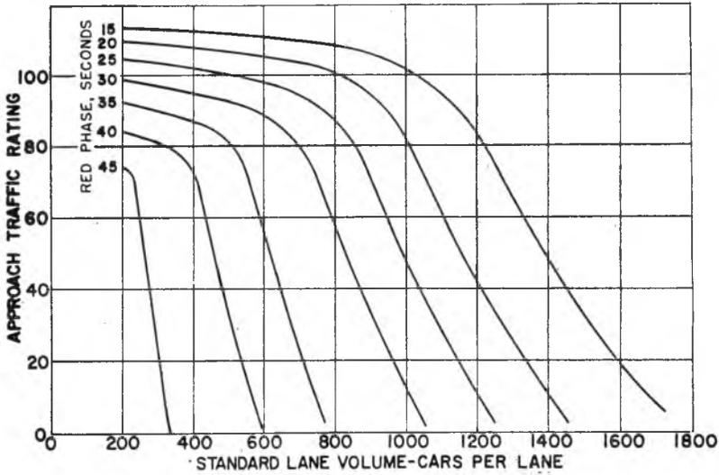
Fig. 11. Intersection approach traffic rating, 60-second cycle and various red phase lengths.
