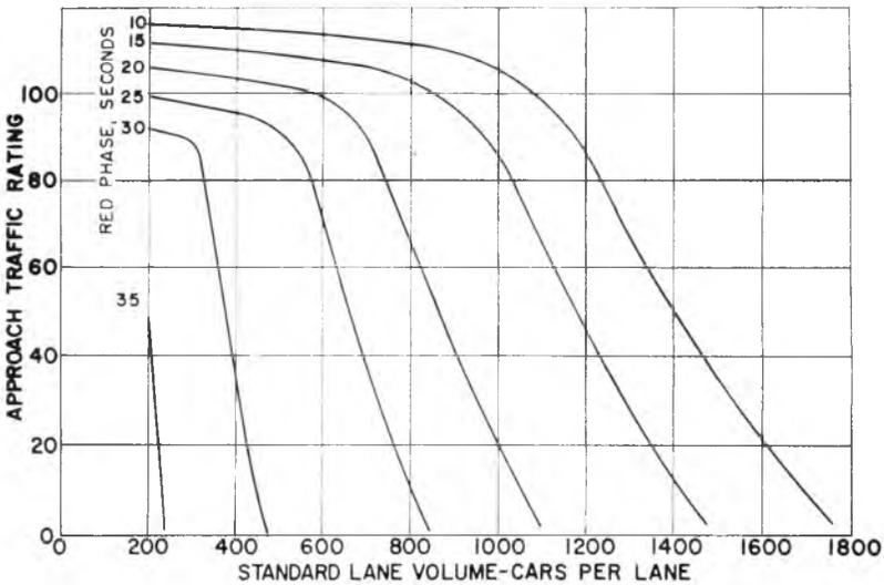
Fig. 8. Intersection approach traffic rating, 45-second cycle and various red phase lengths.
