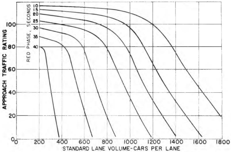
Fig. 10. Intersection approach traffic rating, 55-second cycle and various red phase lengths.
