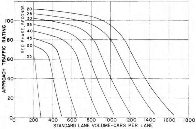
Fig. 13. Intersection approach traffic rating, 70-second cycle and various red phase lengths.
