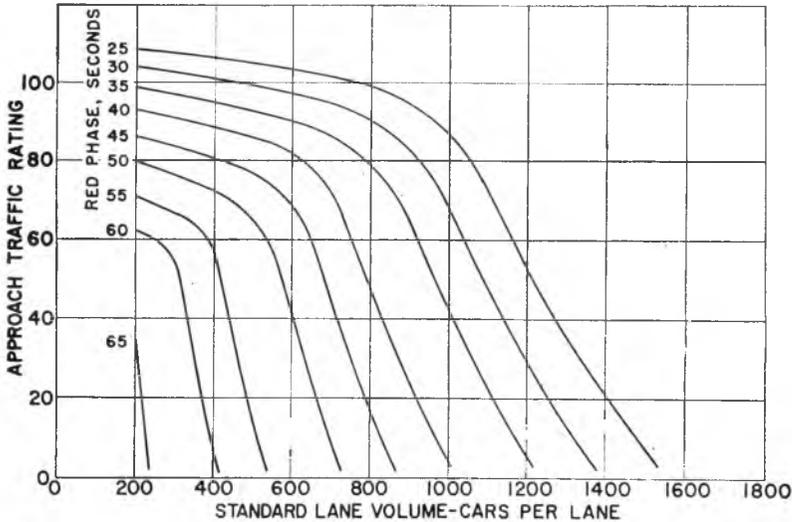
Fig. 15. Intersection approach traffic rating, 80-second cycle and various red phase lengths.
