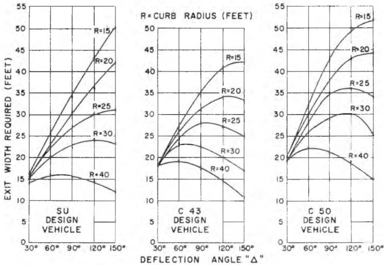
Fig. 4. Required exit widths.
