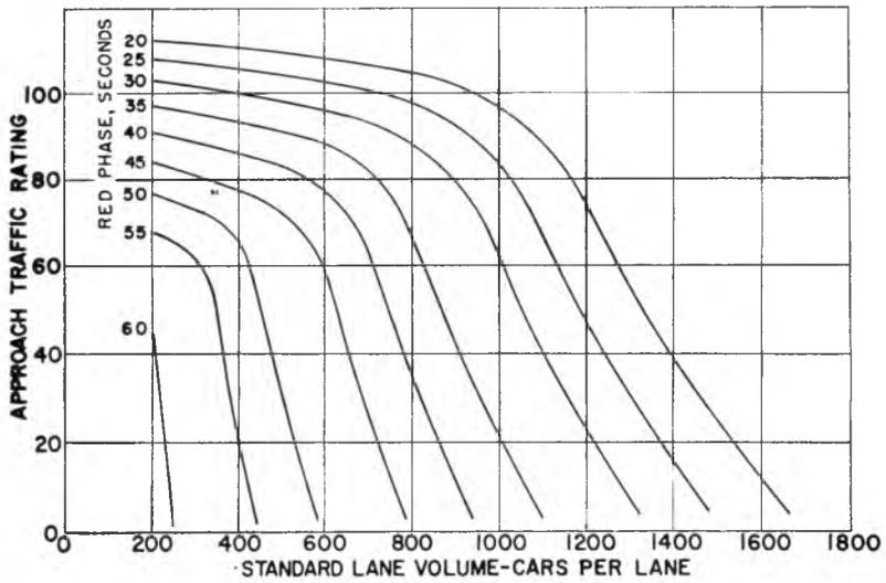
Fig. 14. Intersection approach traffic rating, 75-second cycle and various red phase lengths.
