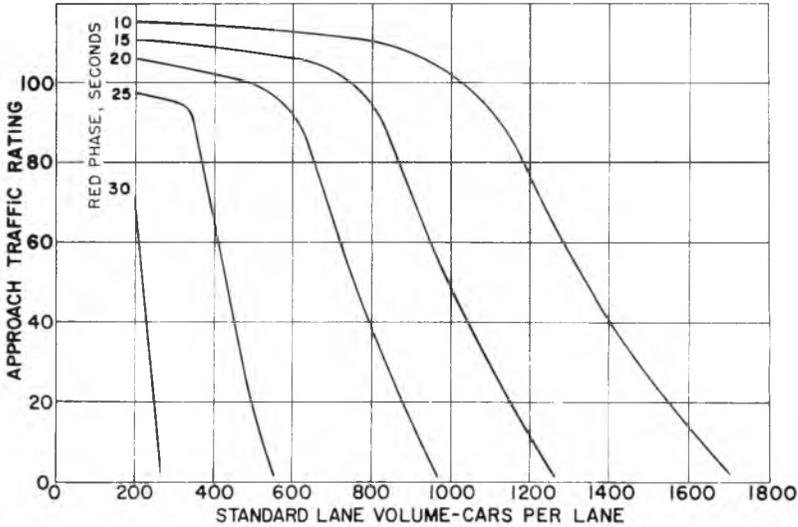
Fig. 7. Intersection approach traffic rating, 40-second cycle and various red phase lengths.
