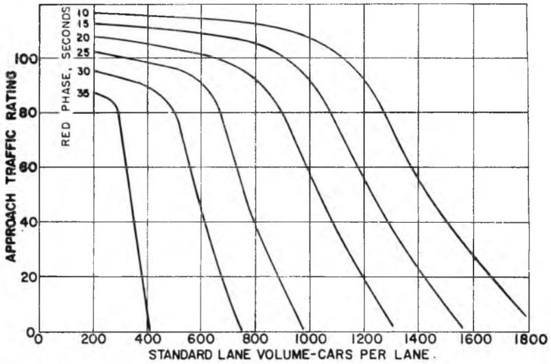
Fig. 9. Intersection approach traffic rating, 50-second cycle and various red phase lengths.
