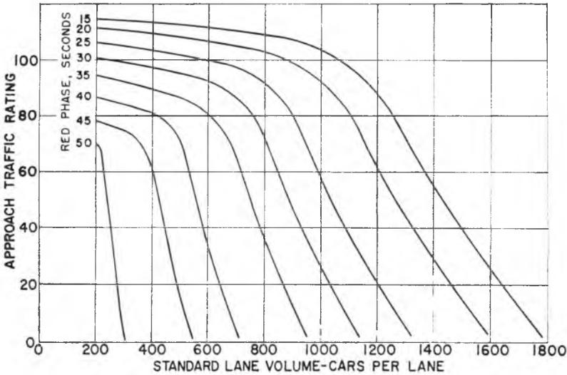
Fig. 12. Intersection approach traffic rating, 65-second cycle and various red phase lengths.
