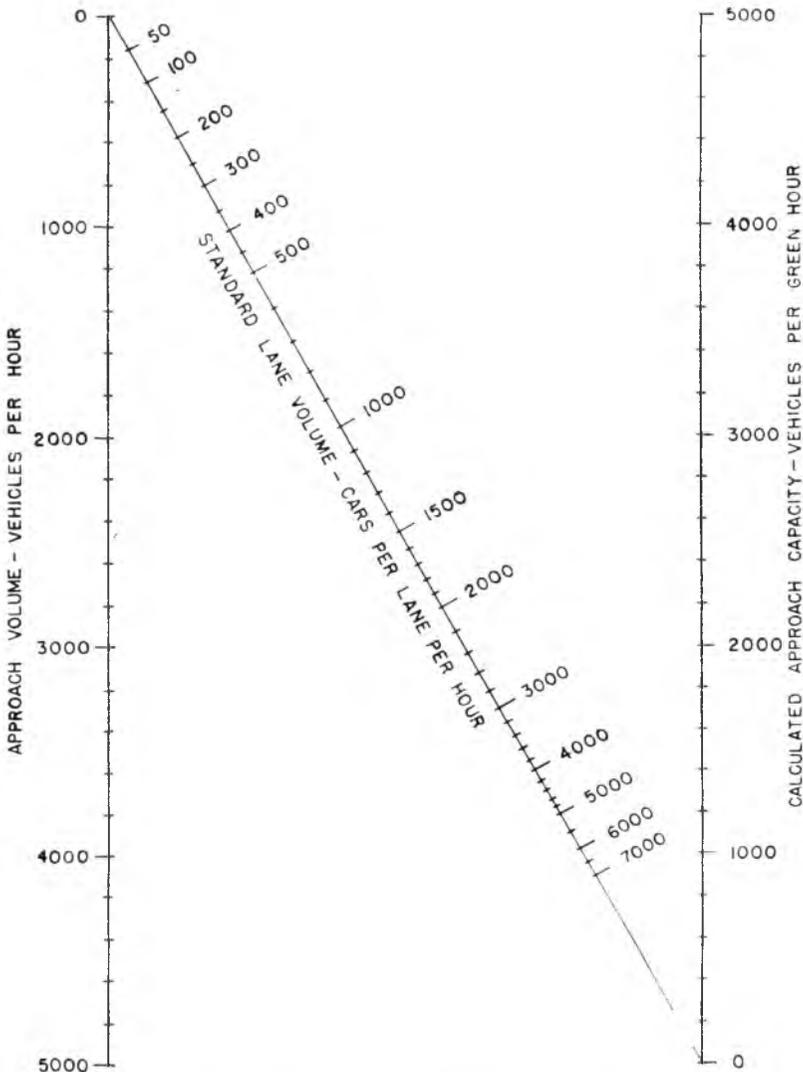
Fig. 16. Determination of standard lane volume.
