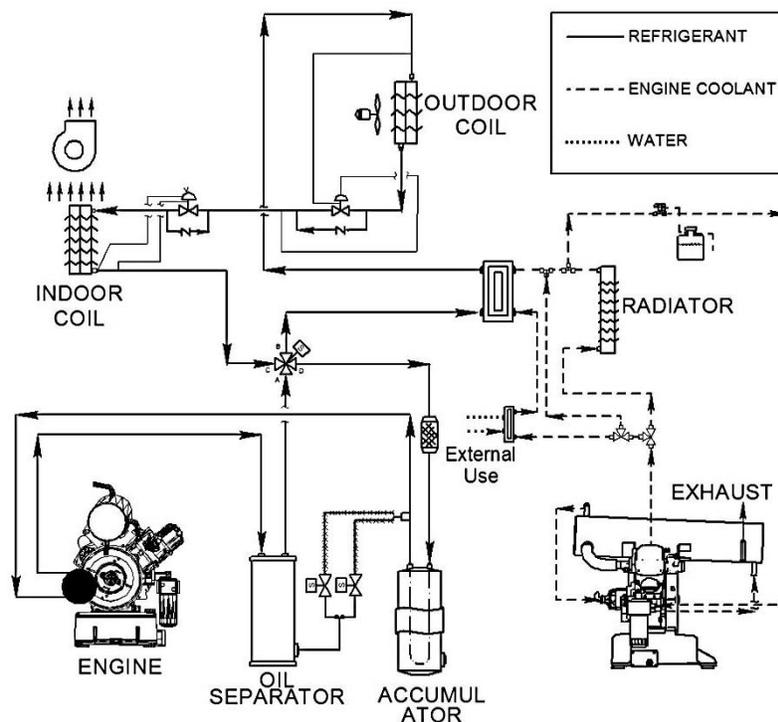
**Figure 1.** GHP schematic; space cooling mode operation shown.
