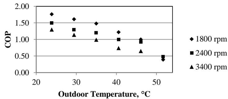
Figure 5. Cooling coefficient of performance of the GHP.
