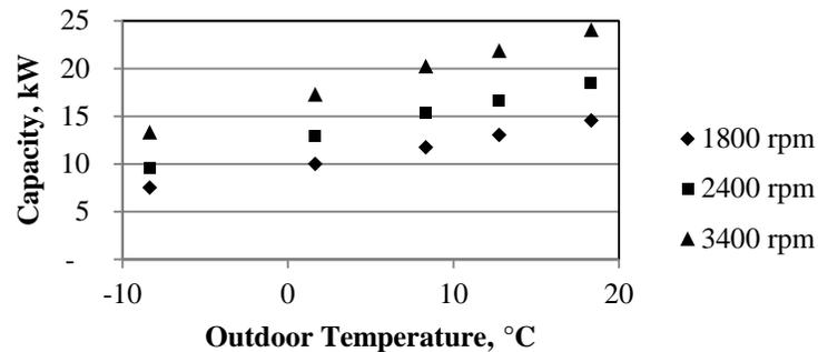
Figure 2. Heating capacity of the GHP at three different speeds.
