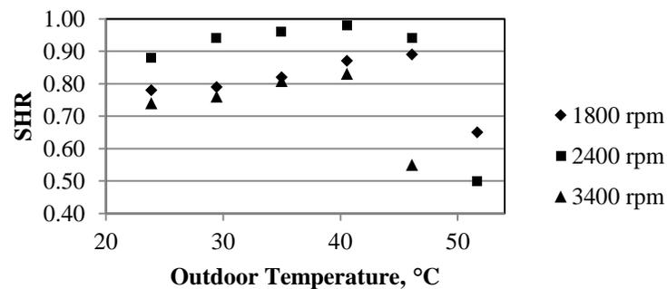
Figure 6. Sensible Heat ratio in cooling mode at different speeds.
