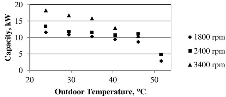
Figure 4. Cooling capacity of the GHP at three different speeds.
