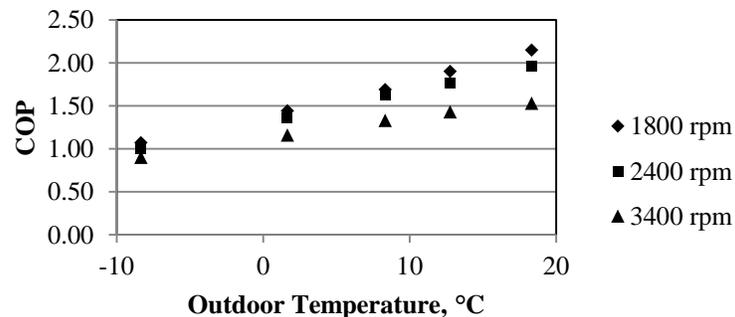
Figure 3. Heating coefficient of performance of the GHP.
