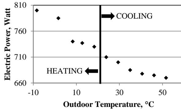
**Figure 7. Electric power consumption of the outdoor unit of the GHP in cooling (right of the vertical line) and heating (left of the vertical line.)**
