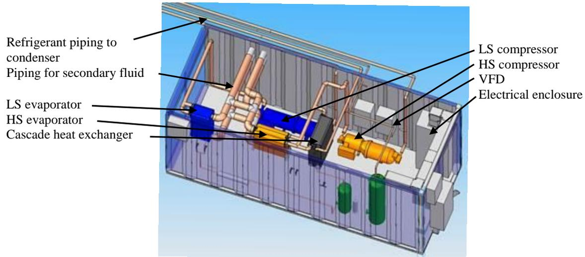
**Figure 2:** Planning and design of the test facility with CAD
