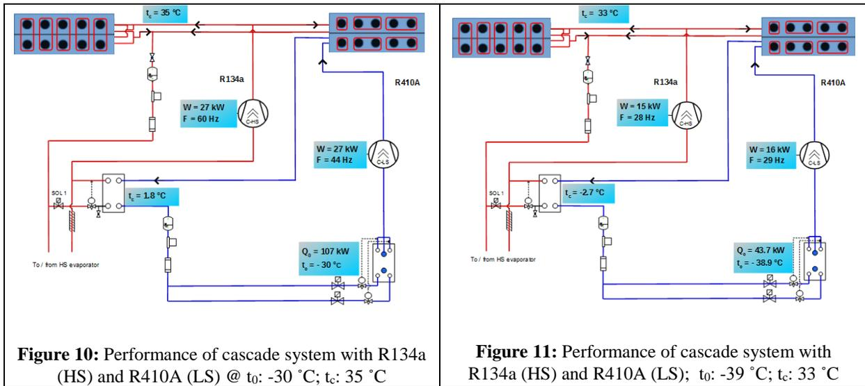
For both tests, the high stage was charged with R134a and the low stage with R410A. The measurement of cooling capacity in Figure 10 is the sum of 100 kW from electrical heater and power of the pump.
