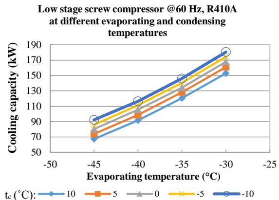
**Figure 6:** Calculated low stage performance (based on manufacturer data)
