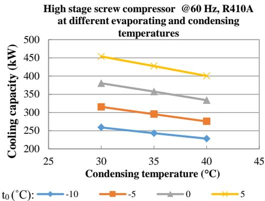
**Figure 5:** Calculated high stage performance (based on manufacturer data)
