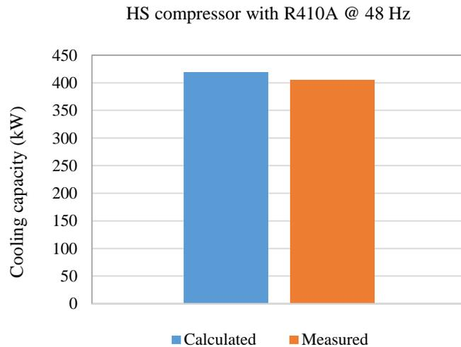
**Figure 12:** Cooling capacity of HS compressor with R410A at  $t_0: 14.6\text{ }^\circ\text{C}$ ,  $t_c: 40\text{ }^\circ\text{C}$
