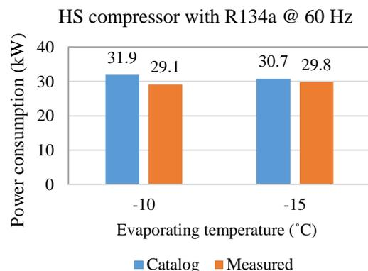
**Figure 9:** Power consumption of HS compressor with R134a at different evaporating temperatures ( $t_c: 35\text{ }^\circ\text{C}$ )
