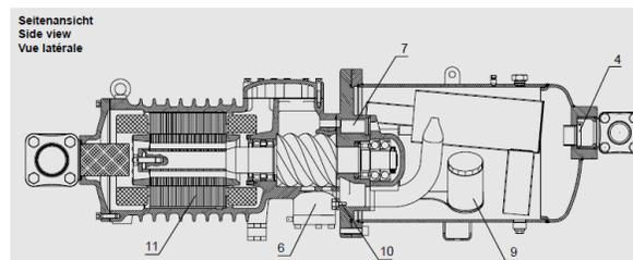
**Figure 7:** Cross-section view of LS or HS screw compressor (4: check valve, 6:Vi-control, 7:differential pressure relief valve, 9: oil filter, 10: discharge temp. control device, 11: built-in motor) (Bitzer Kühlmaschinenbau GmbH)
