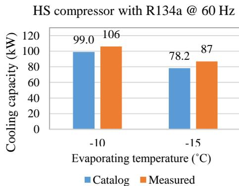
**Figure 8:** Cooling capacity of HS compressor with R134a at different evaporating temperatures ( $t_c: 35\text{ }^\circ\text{C}$ )
