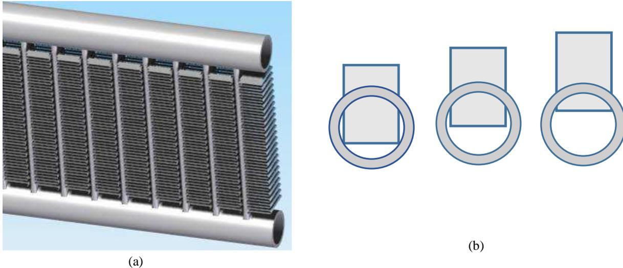
**Figure 1 :** (a) Microchannel heat exchanger assembly; (b) illustration of various microchannel tube insertion lengths into the header.
