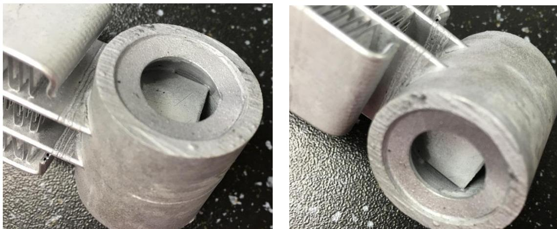
**Figure 7 :** Extensive spreading of liquid filler metal
