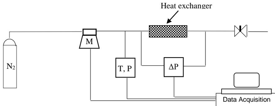
**Figure 3:** Schematic of pressure drop test set-up
