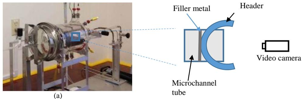
**Figure 4:** lab furnace system for visualization: (a) transparent furnace; (b) schematic of brazing sample assembly
