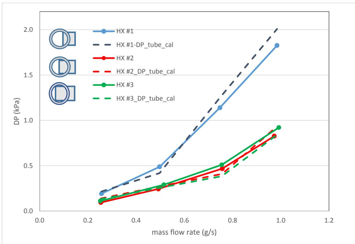
**Figure 5 :** Increased pressure drop for the same nitrogen mass flow rate in HX1 indicates clogged channels and quantifies potential effects in real operation
