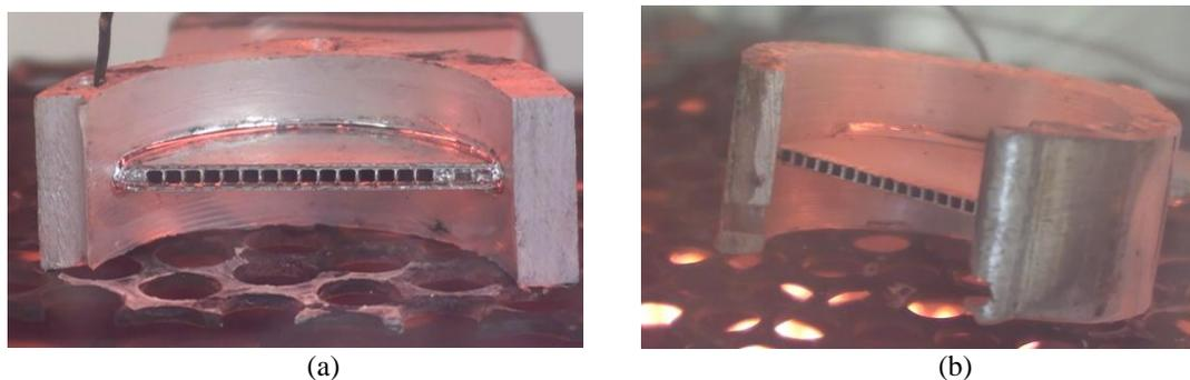
**Figure 8:** Visualization of header/tube brazing process for samples with (a) short tube insertion length, and (b) long tube insertion length.
