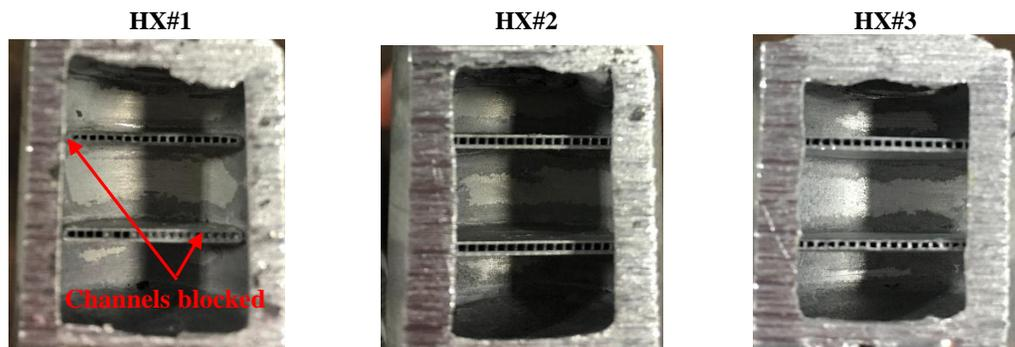
**Figure 6 :** Visual inspection of the microchannel ports in the headers
