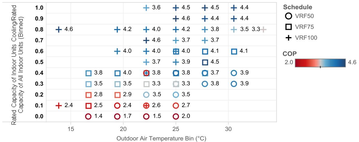
Figure 9: Impact of the rated capacity of active indoor units on efficiency for the VRF system
