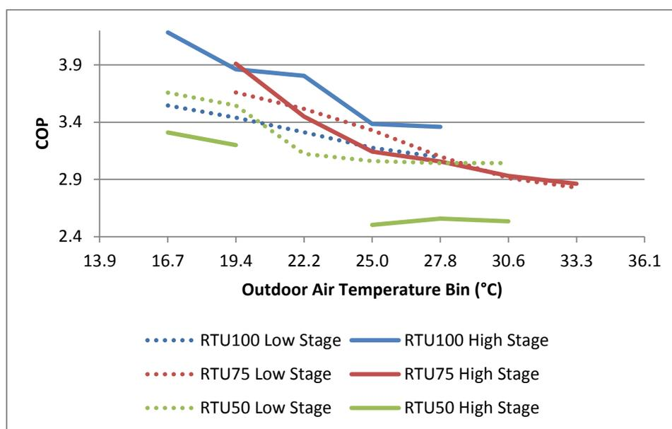
**Figure 8:** Comparison of RTU efficiency during different schedules
