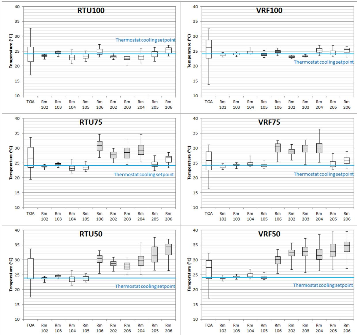
**Figure 4:** Room temperature during RTU and VRF system operation at 100% (top), 75% (middle) and 50% (bottom) load conditions
