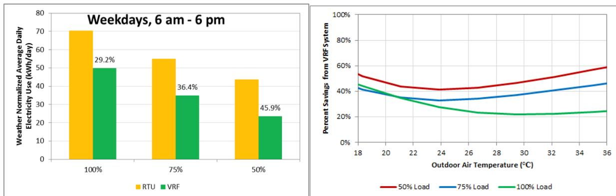
**Figure 6:** Estimated cooling season energy use analysis: (a) total energy use, and (b) energy savings from VRF system
