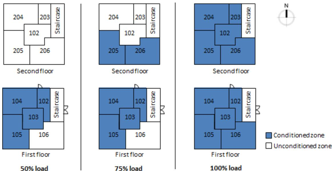
**Figure 3:** Zone conditions to emulate (a) 50% load, (b) 75% load and (c) 100% load
