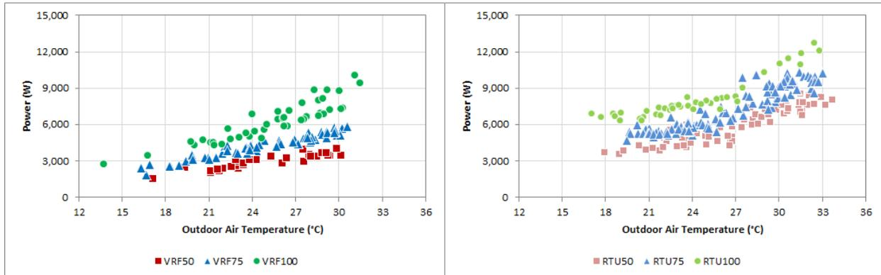
**Figure 5:** Measured power consumption by VRF system (left) and RTU system (right)
