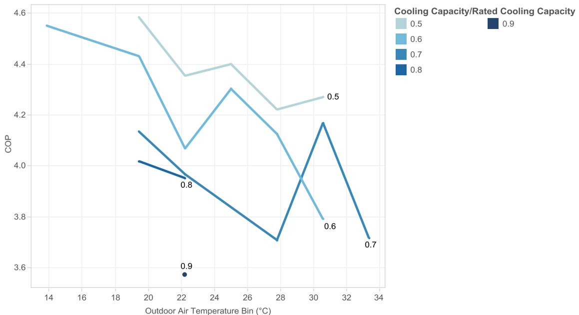
Figure 10: Efficiency of VRF system when most indoor units are providing cooling.
