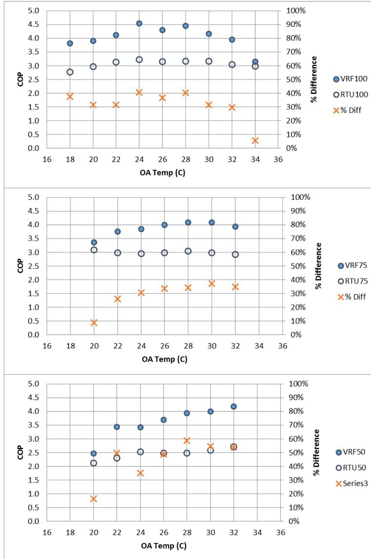
**Figure 7:** COP comparison between RTU and VRF Systems (top: 100% operation; middle: 75% operation; bottom: 50% operation)
