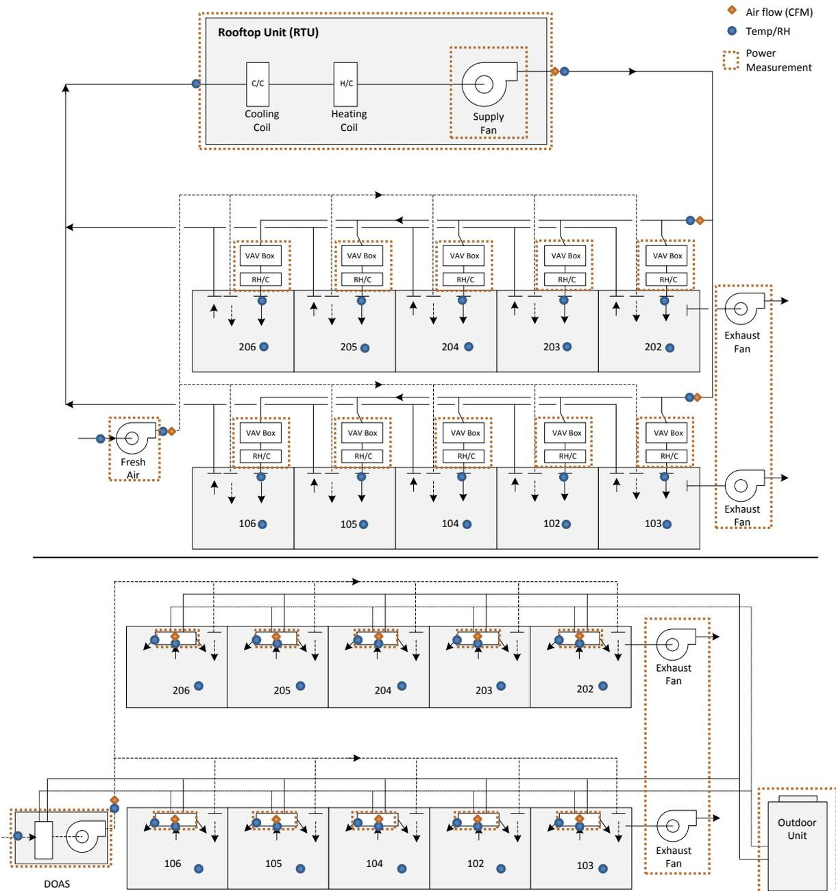
Figure 2: System schematic and monitoring points for RTU system (above) and VRF system (below)
