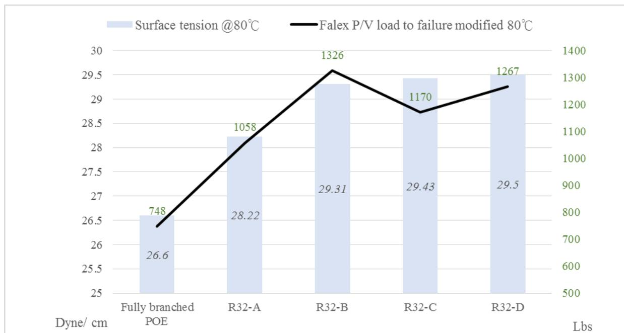
**Figure 3:** Variation of surface tension & extreme pressure properties for ISO-68 oils
