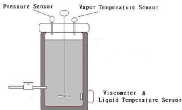
**Figure 2:** Viscosity and solubility test system
