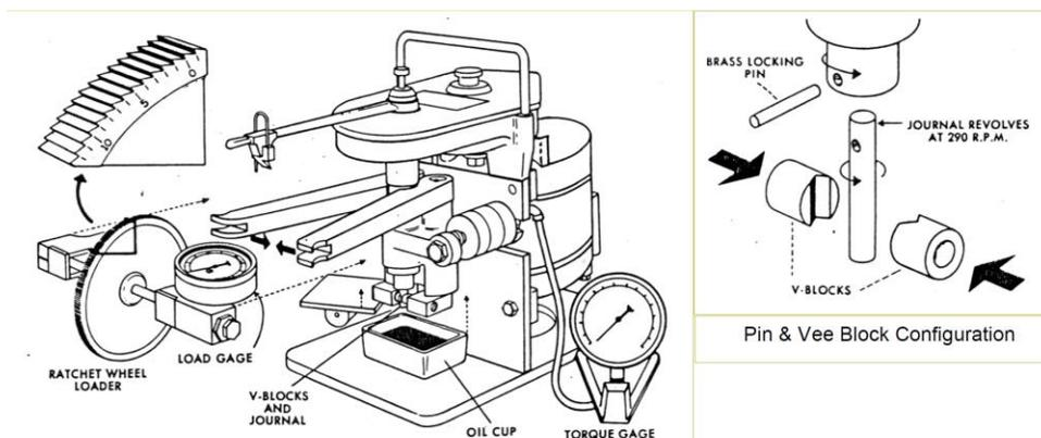
Figure 1: Falex Pin & Vee Block test machine, picture from Falex
