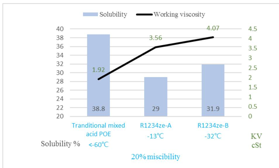
**Figure 7:** Miscibility, solubility and working viscosity of R1234ze refrigeration lubricants (ISO-68)
