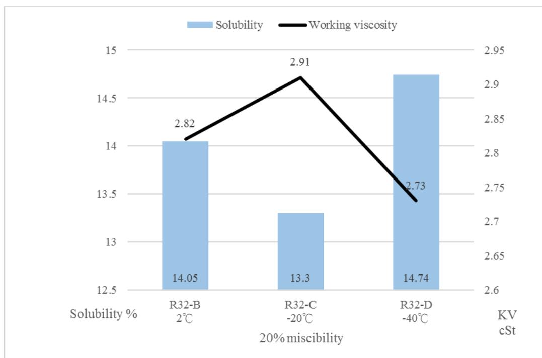
**Figure 5:** Miscibility, solubility and working viscosity of R32 refrigeration lubricants (ISO-68)
