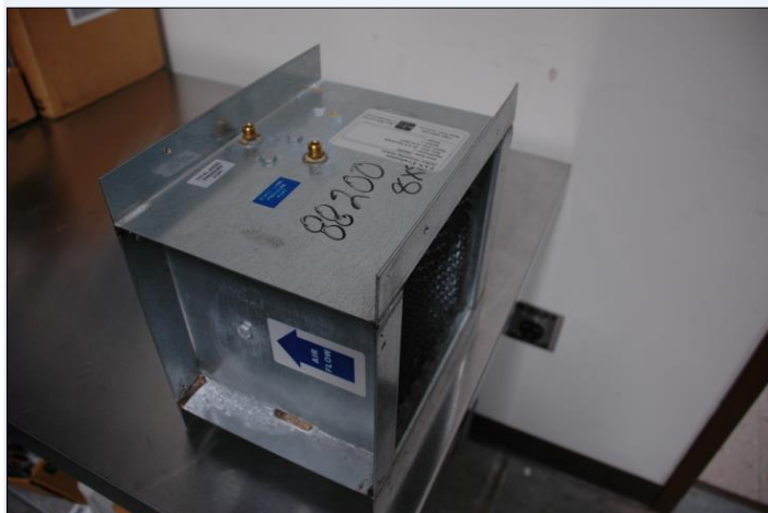
Fig 4. Indoor air flow measurement station.
