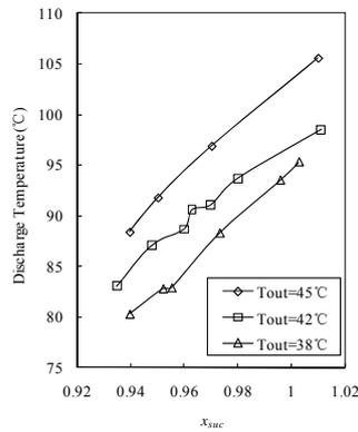
**Figure 5:** The discharge temperature changed with the suction vapor quality
