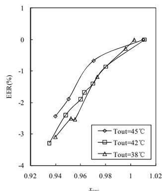
**Figure 3:** The EER changed with the suction vapor quality
