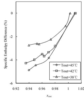
**Figure 6:** The specific enthalpy difference changed with the suction vapor quality
