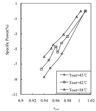
**Figure 7:** The specific power changed with the suction vapor quality
