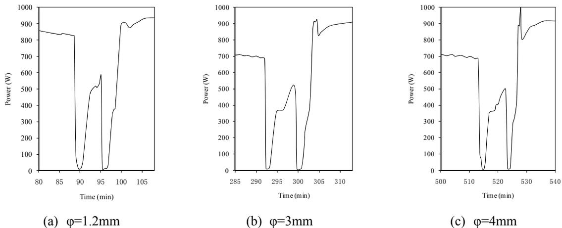
Figure 13: The curves of power under frosting and defrosting
