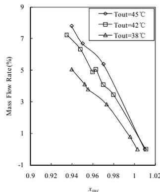
**Figure 8:** The Refrigerant mass flow rate changed with the suction vapor quality
