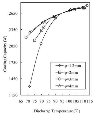
Figure 11: The cooling capacity changed according to discharge temperature
