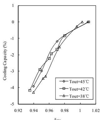
**Figure 2:** The cooling capacity changed with the suction vapor quality
