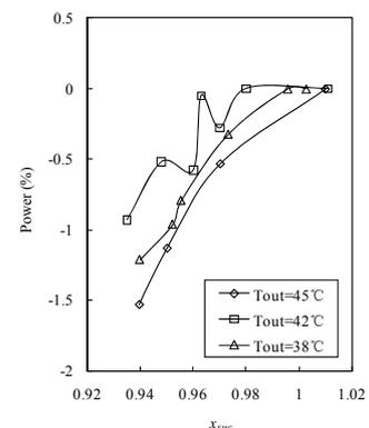
**Figure 4:** The power of conditioner changed with the suction vapor quality
