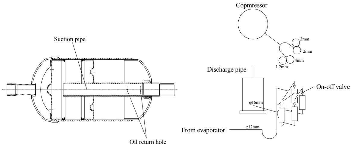
**Figure 9:** Gas-liquid separator and oil return hole**Figure 10:** Four separators installation sketch map
