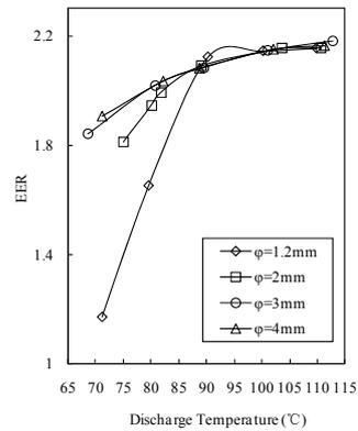
Figure 12: The EER changed according to discharge temperature
