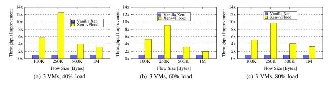
Figure 10: Performance of vFlood with varying load. We fix the number of VMs per core to 3.
