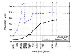
Figure 11: vFlood improvement for different flow sizes
