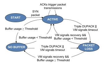
Figure 3: vFlood state machine
