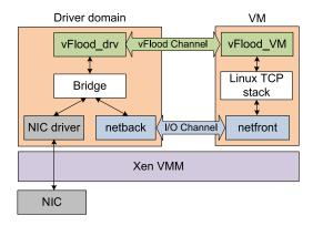
Figure 5: vFlood implementation on Xen
