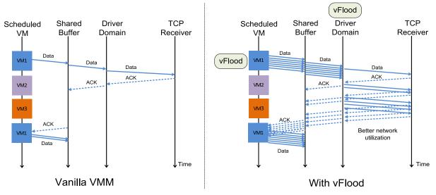
Figure 1: Illustration of TCP connection progress with vanilla VMM and with vFlood-enabled VMM.
