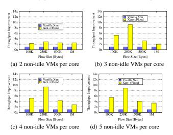
Figure 7: TCP throughput improvement with different number of VMs per core.
