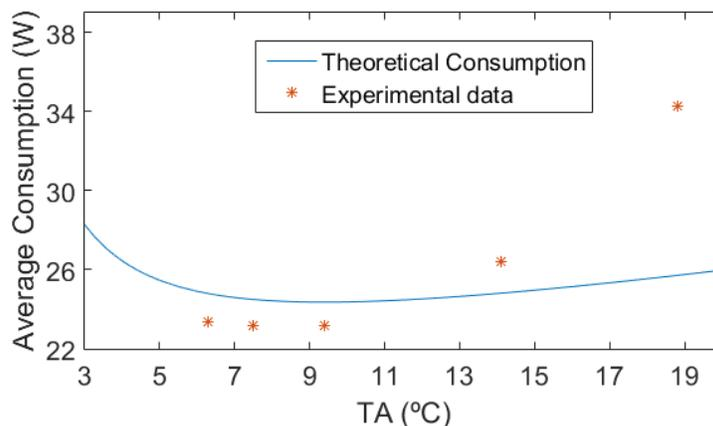
**Figure 8:** Average power consumption - Empty refrigerator
