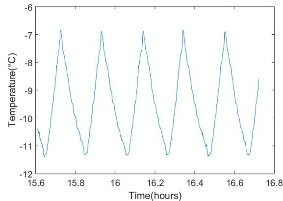
**Figure 2:** Refrigerator cycling operation
