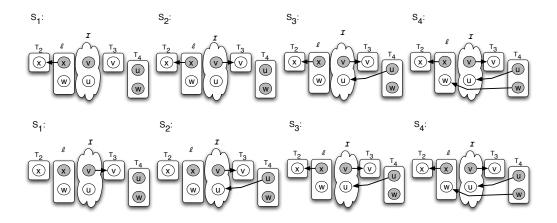
Fig. 12. Serializability of concurrent evaluation means all actions performed by the left-hand side of an isolate can be permuted before the actions performed by the right and *vise versa*.
