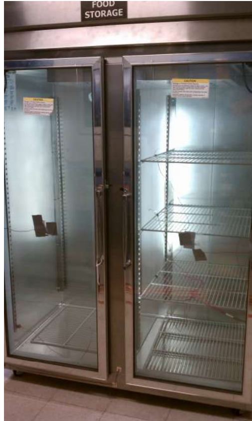
Figure 1: R-404A Reach-in freezer used in experimental testing
