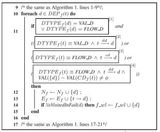
**Algorithm 2:** Optimized Dual Slicing. Edge  $\stackrel{cd}{\longrightarrow}$  denotes control dependence and  $\stackrel{dd}{\longrightarrow}$  denotes data dependence. Method VAL(s) returns the set of value differences reachable from s. Method CD(s) returns the control dependence of s.
