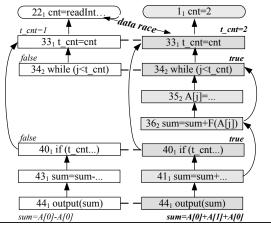
**Figure 5.** The dual slice of the failure in Fig. 4. A symbol  $s_i$  represents the ith instance of statement s in the trace.
