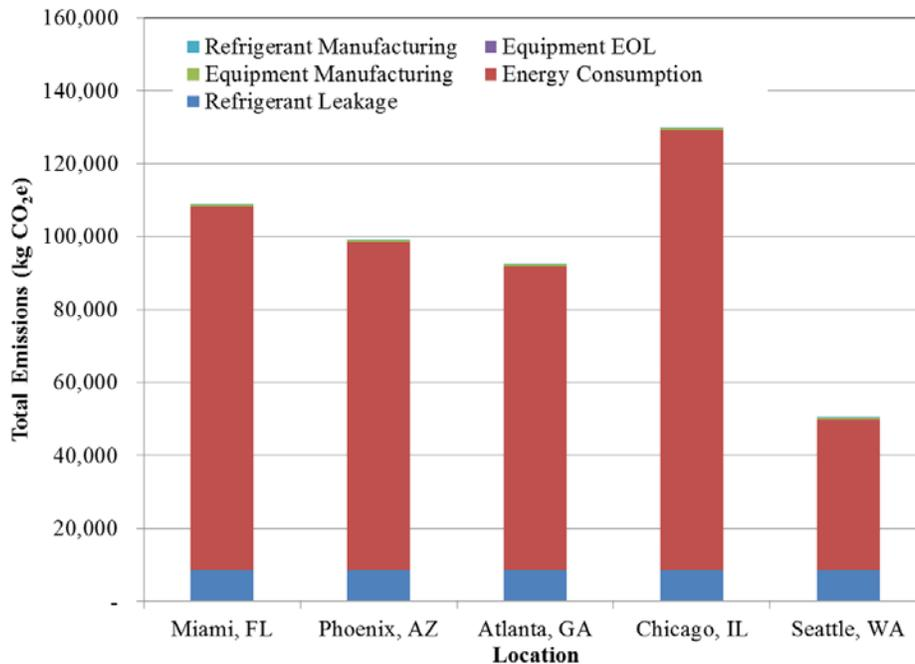
**Fig. 1:** LCCP Comparison for Residential Heat Pump Sample
