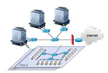
Fig. 3. Example of an enterprise campus network.
