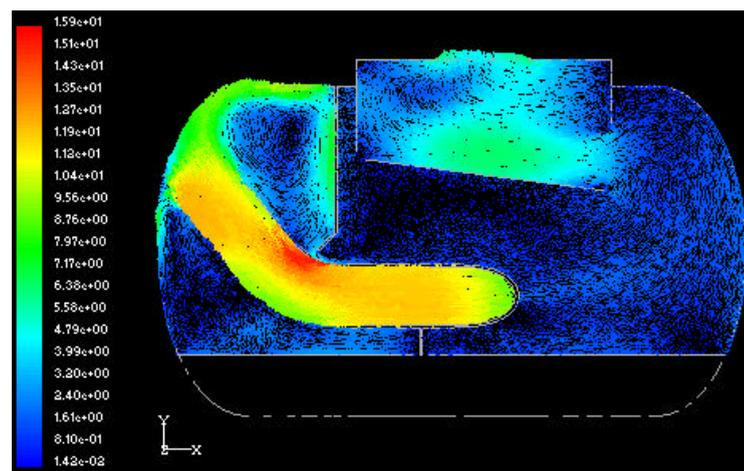
figure 3 velocity vector in the oil vessel (m/s)
