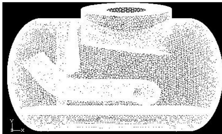
fig 2 unstructured mesh of the original oil vessel
