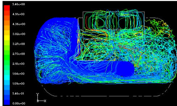
figure 8 track curve of oil droplets in the new oil vessel (m/s)
