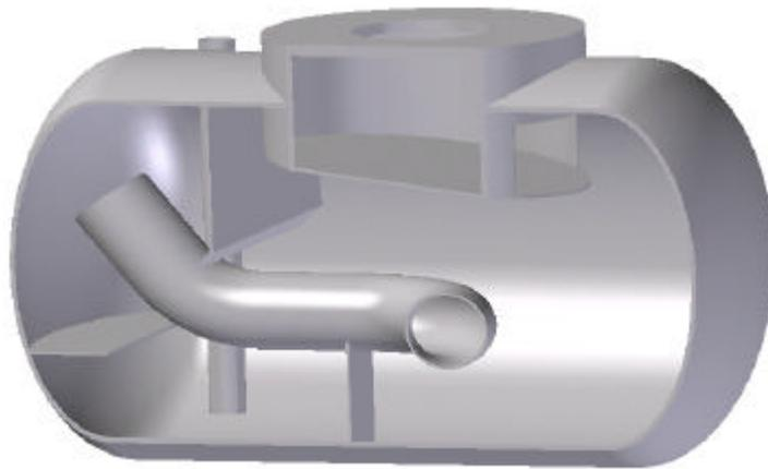
fig 1 solid model for the original oil vessel
