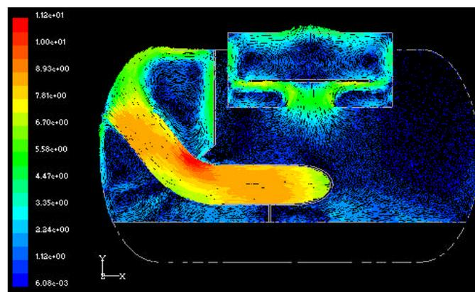
figure 7 velocity vector in the new oil vessel (m/s)
