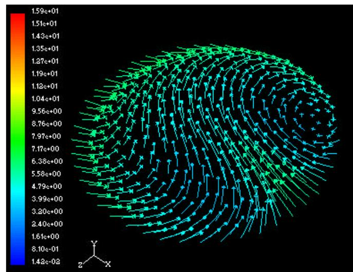
figure 5 velocity vector at the outlet (m/s)
