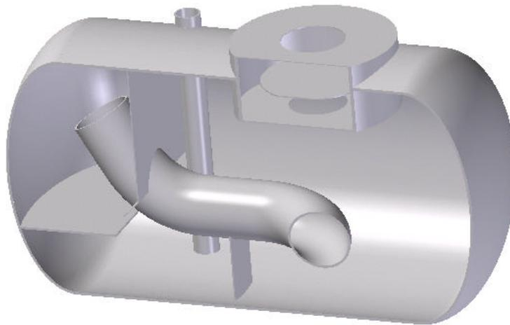
figure 6 solid model for new oil vessel
