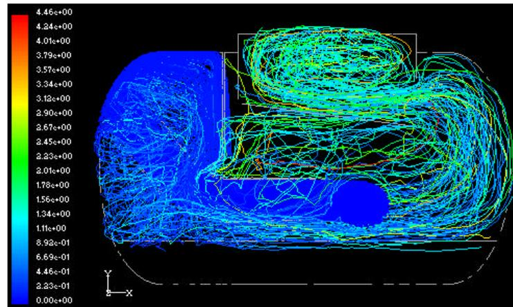
figure 4 track curve of oil droplets in the oil vessel (s)
