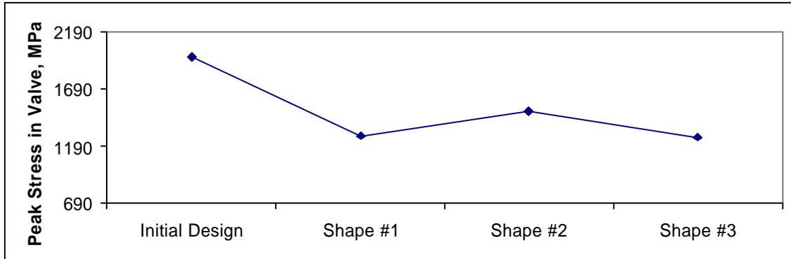
Figure 5. Stress Improvement in the CO<sub>2</sub> Compressor Discharge Valve by Shape Optimization
