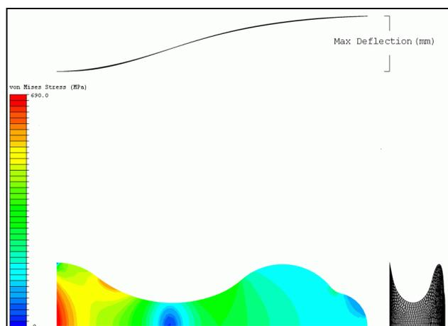
Figure 4. Final CO<sub>2</sub> Suction Valve Design
