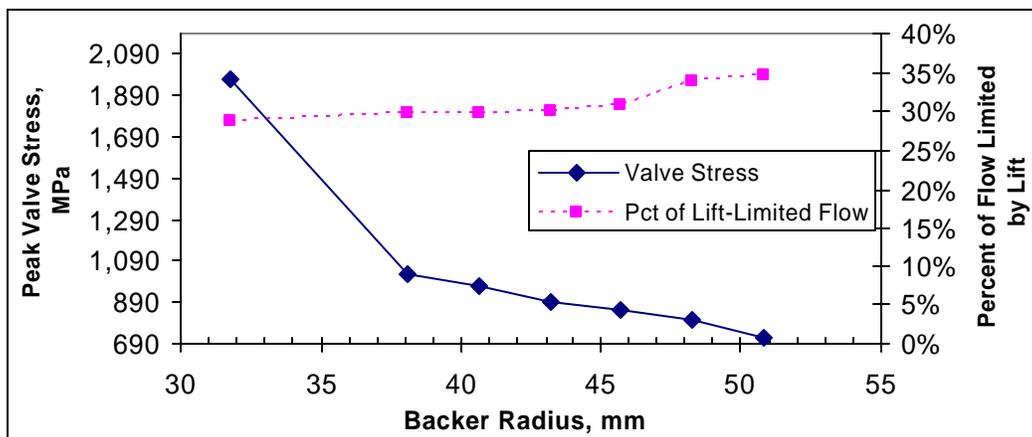
Figure 6. Iteration of Discharge Backer Radius for a Successful Valve Design
