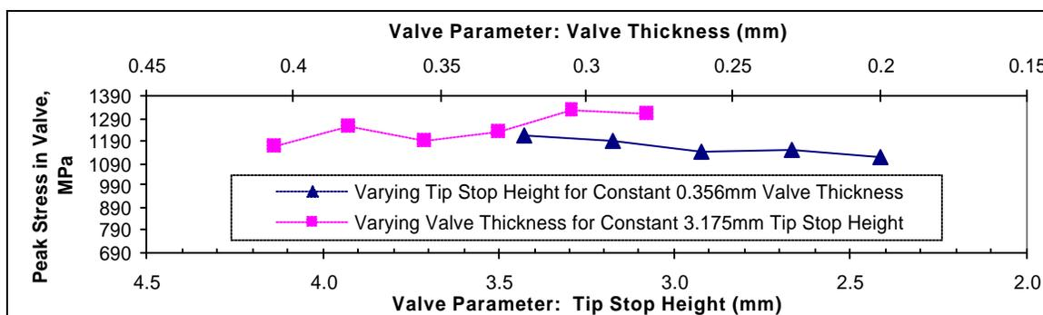
Figure 1. Initial choice of iterated parameters for suction valve stress improvement.
