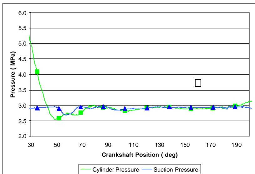
Figure 8. Cylinder Pressure vs. Suction Plenum Pressure
