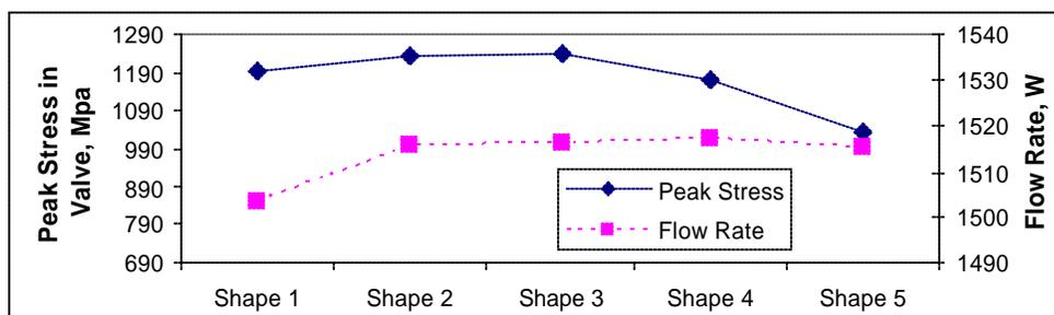
Figure 2. Improvement in Valve Stress Achieved through Shape Modification
