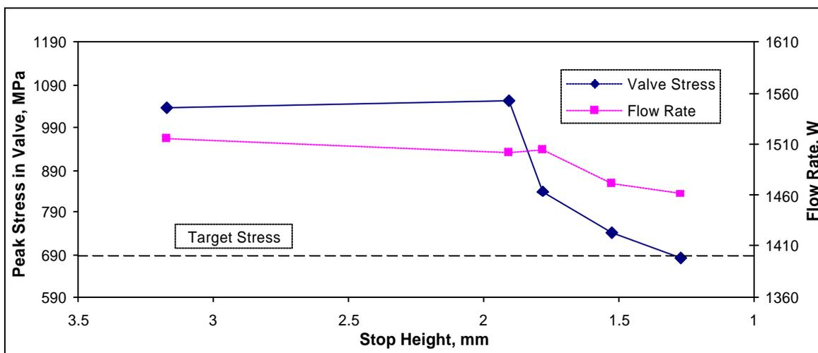
Figure 3. Iteration of Tip Stop Height on the Optimal Suction Valve Shape
