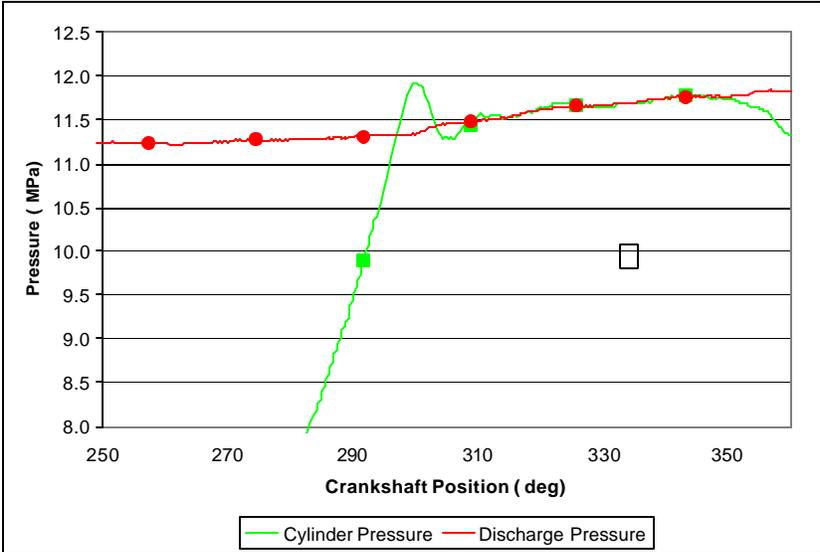
Figure 9. Cylinder Pressure vs. Discharge Plenum Pressure
