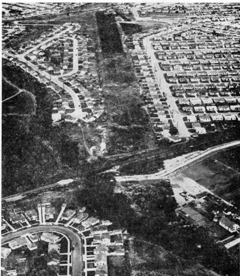
Fig. 5. Illustration of how subdividers cooperated in the design of the East Shore Freeway in Alameda County, California, a highway designed to handle a large volume of traffic going through Oakland. None of the adjacent residences have direct access to the freeway; it was planned that way.
