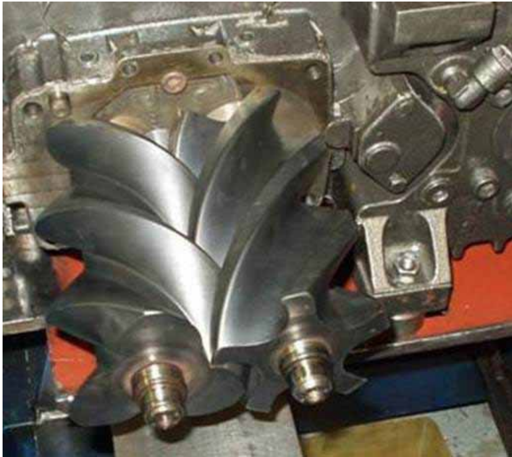
Figure 6: Compressor rotors, housing removed
