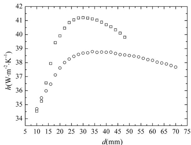
**Figure 8:** Effect of the distance between the emitter electrodes  $d$  on heat transfer coefficient.  $T_{plate}=343.15 \text{ K}$ ,  $U_0=4.5 \text{ kV}$ ,  $u_0=0.28 \text{ m}\cdot\text{s}^{-1}$ . □, ionic wind with two emitter electrode; ○, ionic wind with three emitter electrode.
