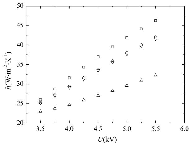
**Figure 4:** Heat transfer coefficient at different horizontal distance between the emitter electrode and the collector  $G$ , plate temperature is  $343.15$  K. □,  $G=0$  mm; ○,  $G=2$  mm; ▽,  $G=4$  mm; △,  $G=6$  mm.
