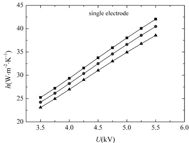
**Figure 5:** Heat transfer coefficient at different plate temperature. ■, plate temperature is 343,15 K; ●, plate temperature is 333,15 K; ▲, plate temperature is 323,15 K.
