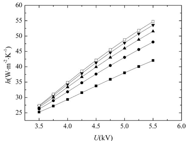
**Figure 7:** Influences of the electrode numbers on force convection of horizontal flow. ■, single emitter electrode; ●, two emitter electrodes; ▲, three emitter electrodes; ▼, four emitter electrodes; □, five emitter electrodes.
