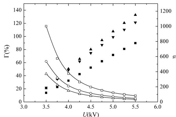
**Figure 10:** Percentage improvement in average heat transfer and cooling effectiveness of the horizontal ionic wind. ■, percentage improvement in average heat transfer of ionic wind with single electrode; ▼, percentage improvement in average heat transfer of ionic wind with two electrodes; ▲, percentage improvement in average heat transfer of ionic wind with three electrodes; □, cooling effectiveness of the horizontal ionic wind with single electrode; ○, cooling
