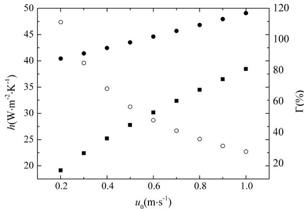
**Figure 9:** Effects of the inlet velocity of bulk flow  $u_0$  on heat transfer coefficient. ■, heat transfer coefficients of bulk flow; ●, heat transfer coefficients of bulk flow with ionic wind; ○, percentage improvement in average heat transfer coefficient.
