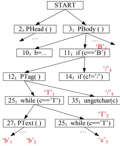
**Figure 4: Execution Trace and Control Dependence Graph.**
