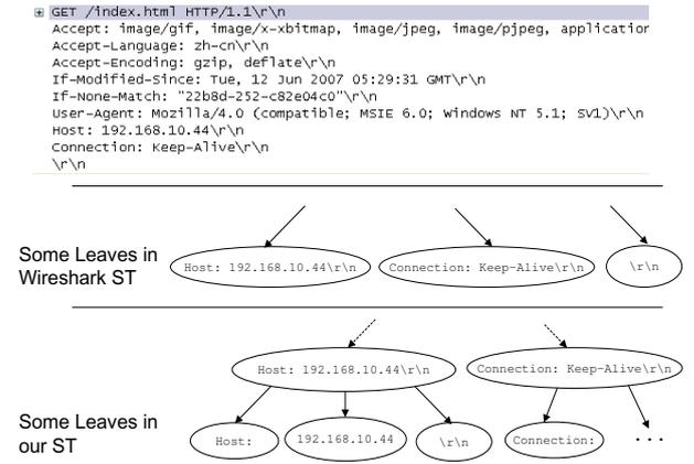
**Figure 9: Tree Comparison Between Wireshark and Ours for apache.**
