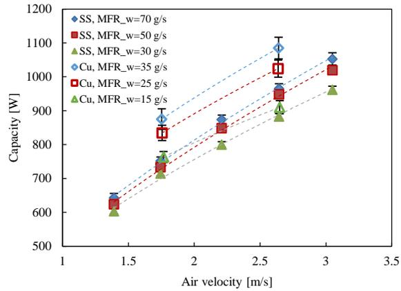
**Figure 12:** Effects of air velocity on capacity for different water flow rates for SSHX and CuHX
