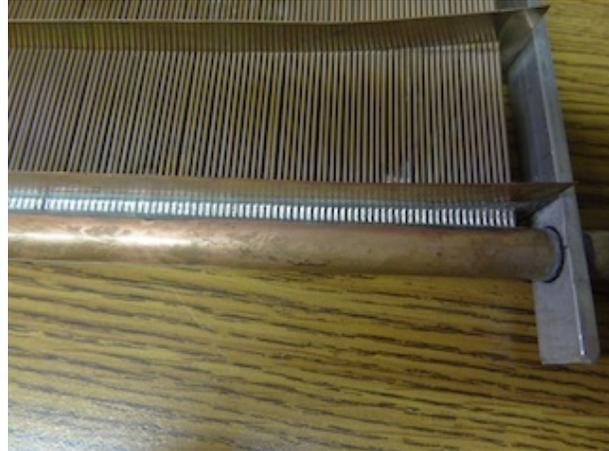
**Figure 4:** Soldered section between spacer and manifold
