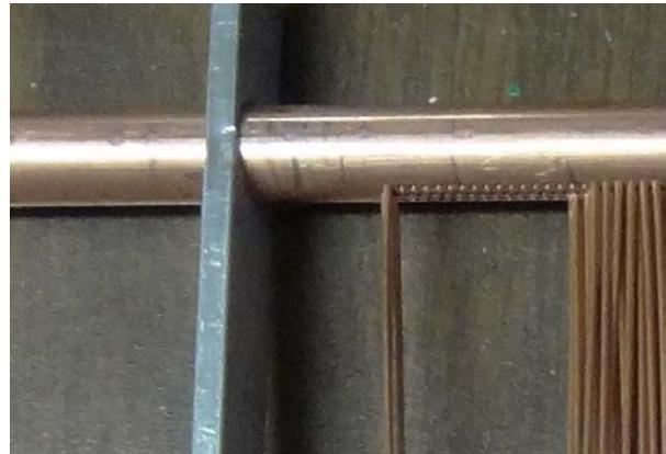
**Figure 2:** Tubes inserted into opposite manifold
