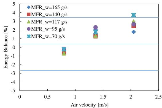
**Figure 14:** Energy balance between air and water for CuHX-10kW
