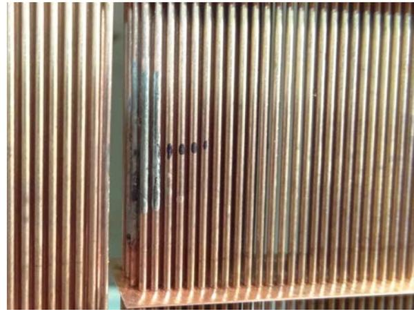
**Figure 10:** Repaired leak in tube.
