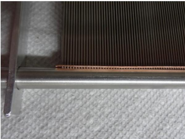
**Figure 5:** Stainless tubes and manifolds
