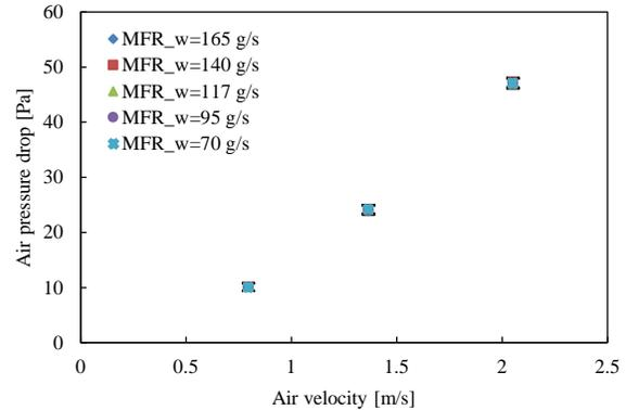
**Figure 16:** Effects of air velocity on air pressure drop for different water flow rates for CuHX-10kW
