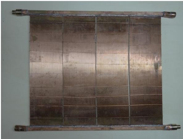
**Figure 9:** Completed 10kW heat exchanger with fittings
