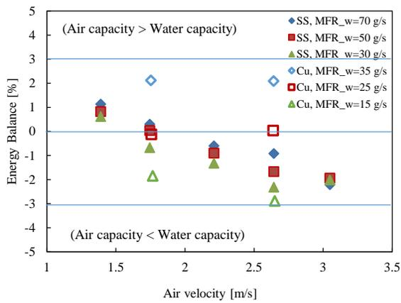
**Figure 11:** Energy balance between air and water for SSHX and CuHX
