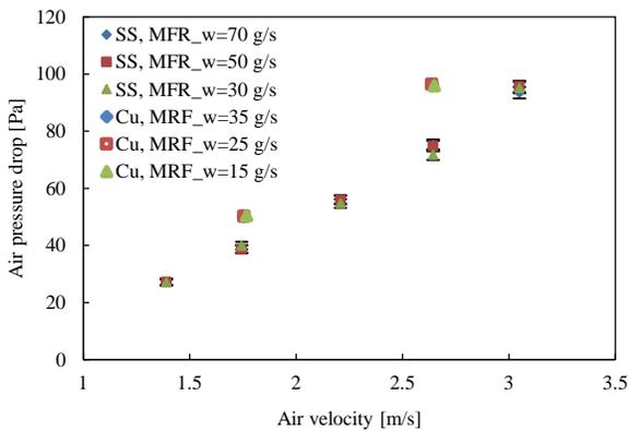
**Figure 13:** Effects of air velocity on air pressure drop for different water flow rates for SSHX and CuHX
