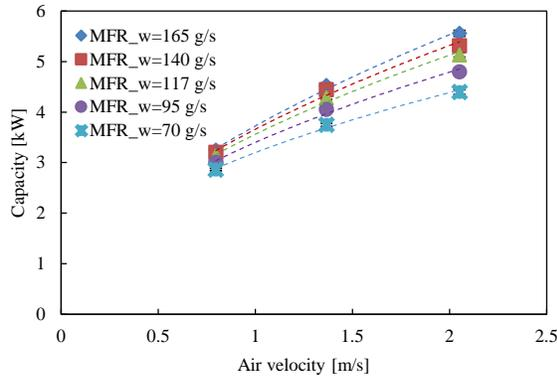
**Figure 15:** Effects of air velocity on capacity for different water flow rates for CuHX-10kW
