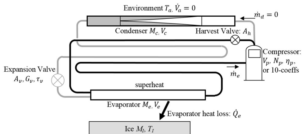
**Figure 3:** Ice machine model operating in harvest mode.
