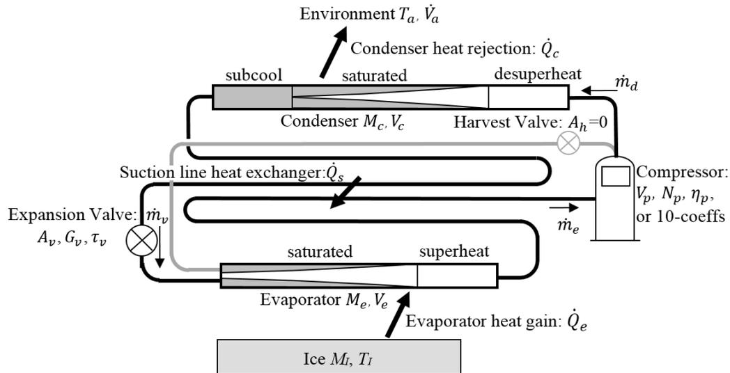
**Figure 2:** Ice machine model operating in freeze mode.
