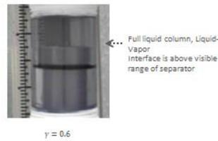
**Figure 8:** Separator 2,  $P = 115$  Psia [800 kPa]  $\dot{m}_T = 6$  lbm/hr [2.7 kg/hr]
